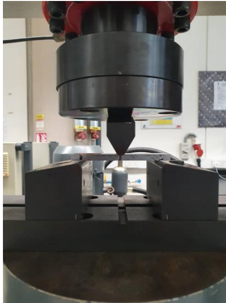
Figure 3.6: Three point bending test
