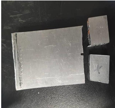
Figure 3.8: Sectioning of Aluminium 7075
