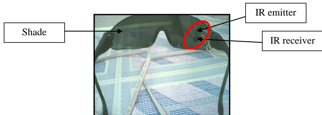
Figure 25: IR Transmitter and receiver at the corner of the shade
