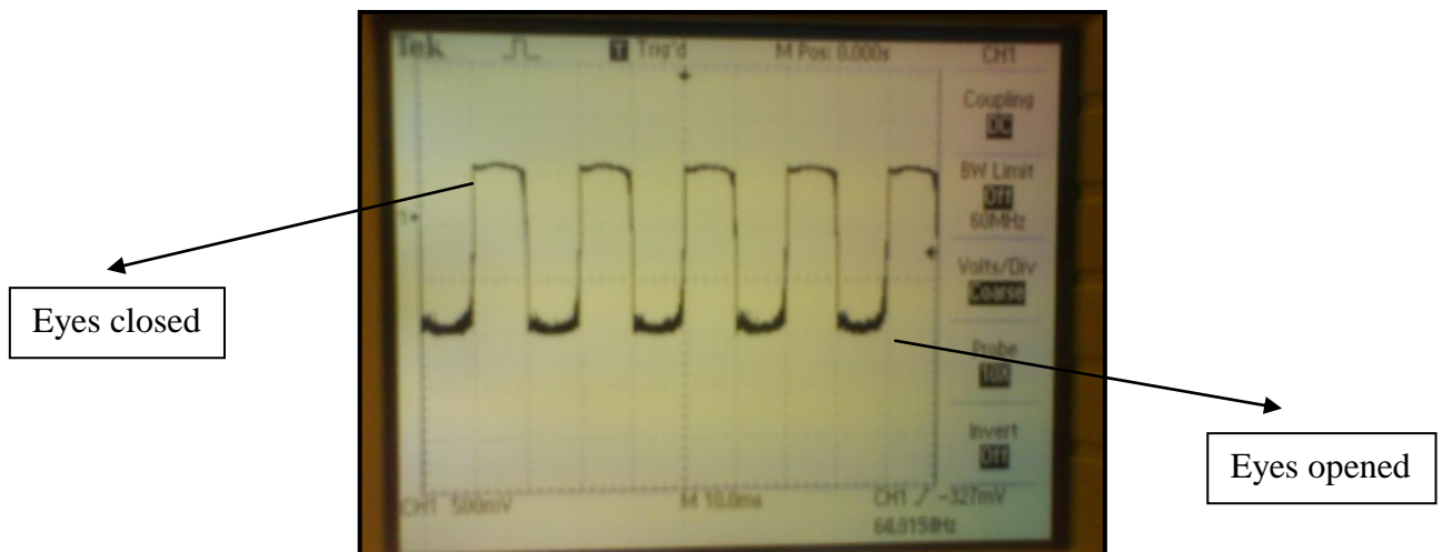
Figure 20: Output voltage of the IR receiver from digital oscilloscope
