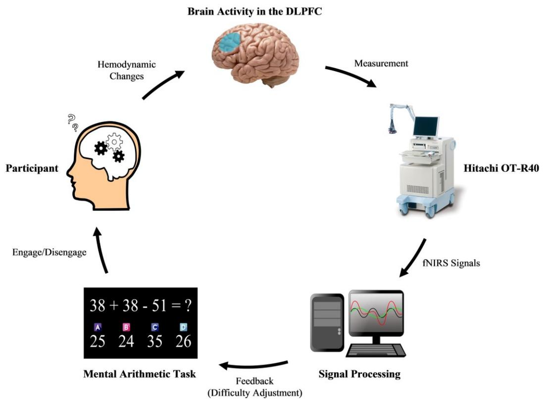
Figure 3.2: The schematic diagram of the fNIRS-DDA system.
