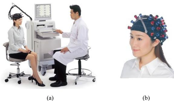
Figure 2.9: Hitachi ETG-4000 fNIRS system in use. (b) A participant wearing a probe holder that holds all the probes in place.
