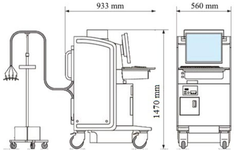
Figure 3.3: OT-R40 has dimensions of 560 mm (length) × 933 mm (width) × 1470 mm (height).
