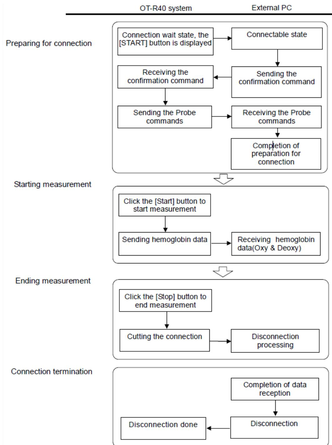
Figure 3.6: Flowchart for sending and receiving fNIRS data between computer and OT-R40 in real time.
