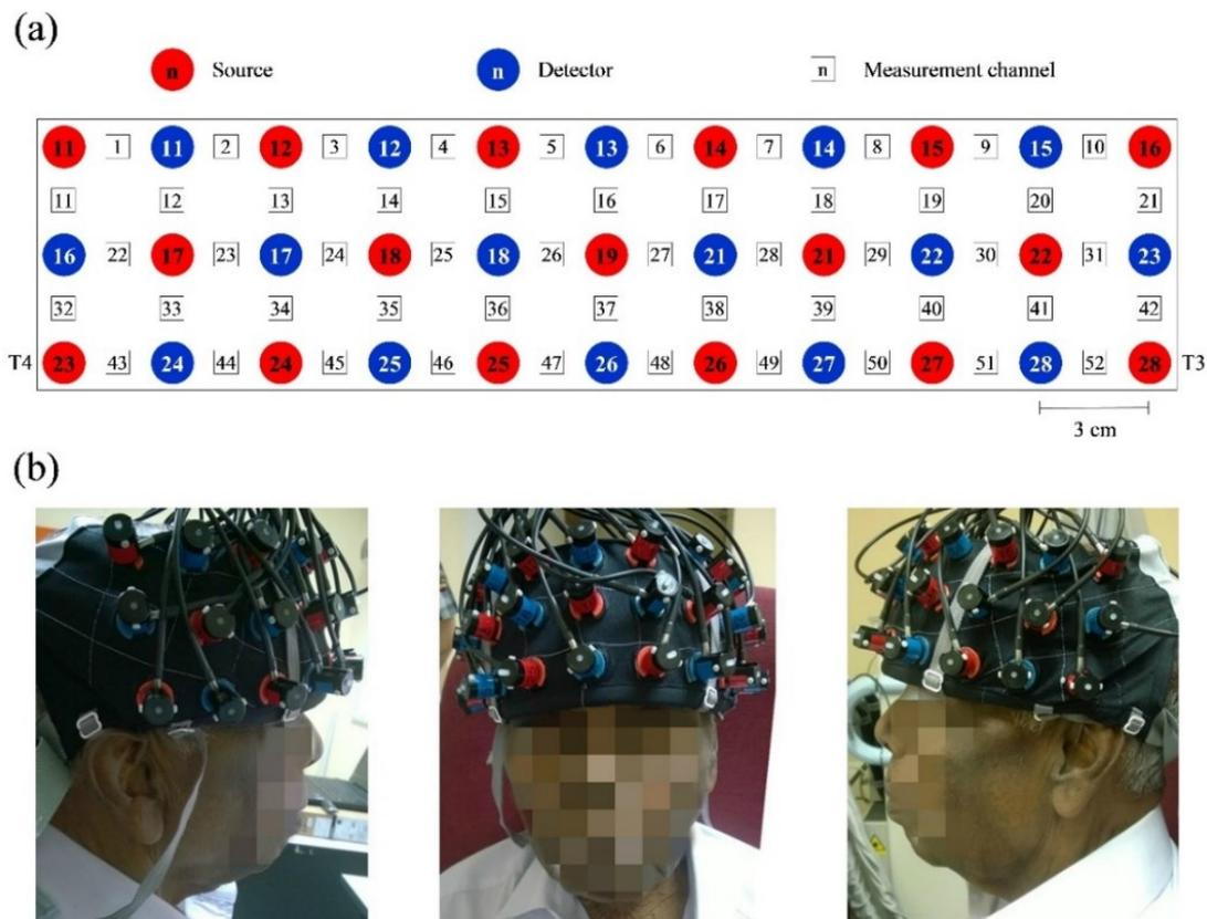
Figure 3.5: Details regarding the probes and measurement channels. (a) 17 emitters and 16 detectors are arranged in such way to form 52 measurement channels. (b) Emitter 23 and 28 are placed directly at T4 and T3 respectively. Such arrangement is sufficient to measure the entire prefrontal cortex including DLPFC.
