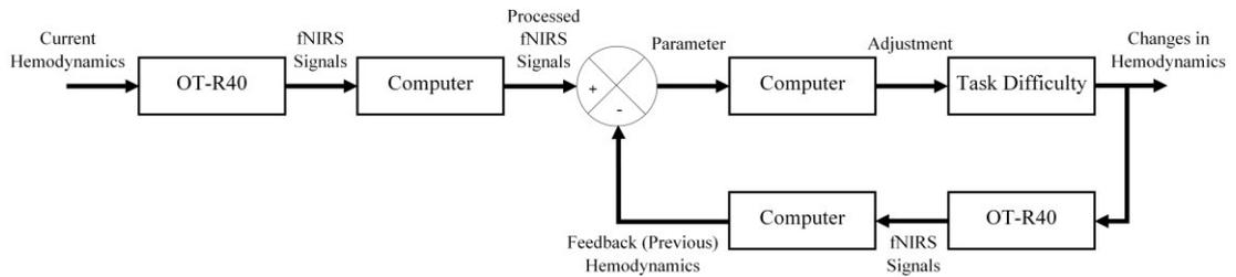
Figure 3.1: The fNIRS-DDA's closed-loop feedback control system block diagram.
