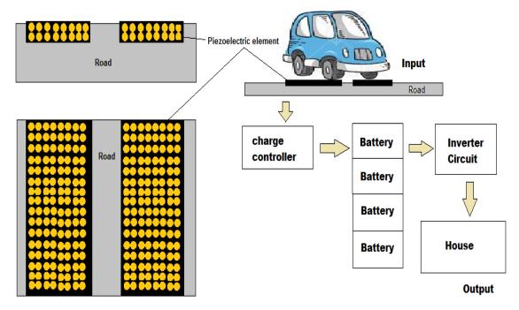
Figure 7: Design Highway Power Harvester
