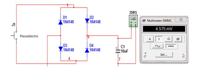
Figure 9: Schematics diagram piezoelectric circuit
