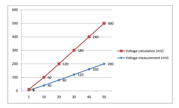
Figure 14: Force 500 Newton for 50 piezoelectric
