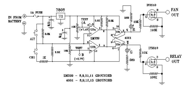
Figure 4: Schematics of charge controller [4]
