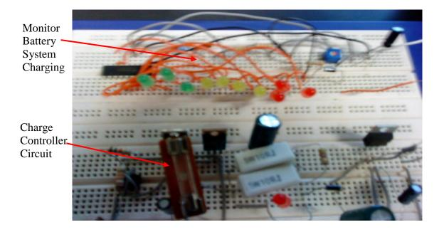
Figure 16: Charge controller circuit and Monitor Battery system
