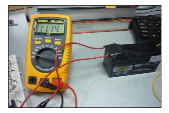
Figure19: Voltage Input
