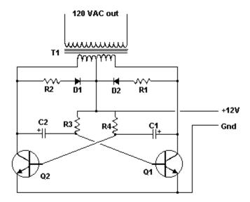
Figure 5: Schematics of Inverter [5]
