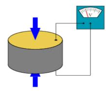
Figure 2: A piezoelectric disk generates a voltage when deformed. [6]
