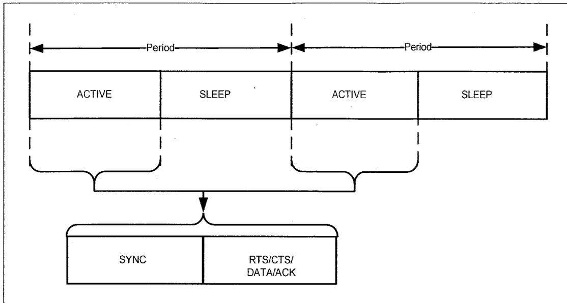
Figure 2.2 SMAC alternatively turns ON and OFF the radio in active and sleep period adopted by [38]
