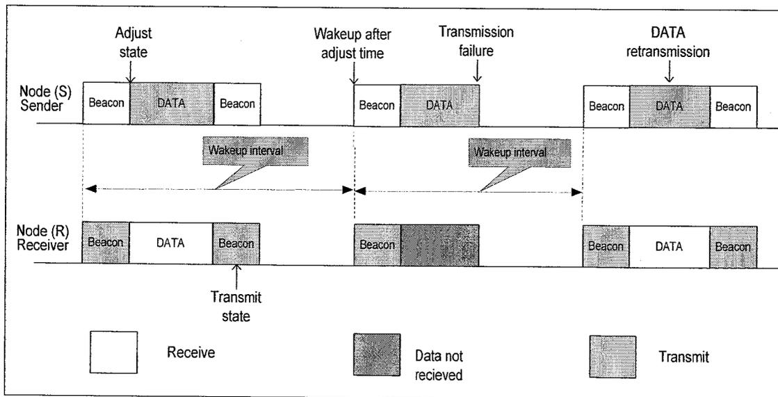
Figure 2.9 PW-MAC predictive-wakeup mechanisms for transmission referred by [43]
