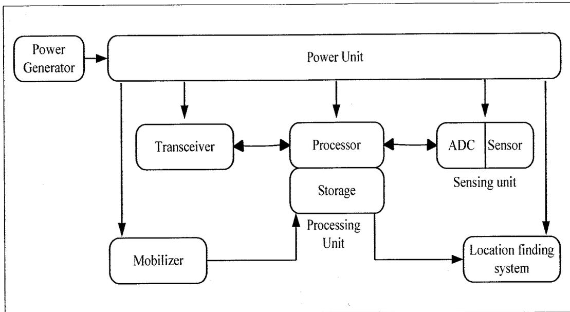
Figure 1.2 Basic architecture of a wireless sensor node
