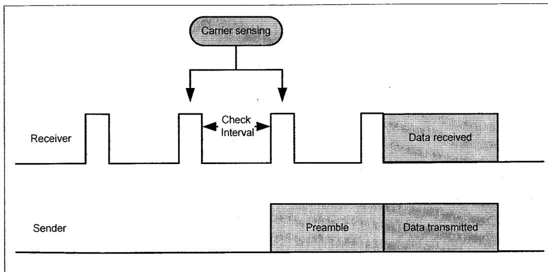
Figure 2.5 B-MAC introduces preamble for transmission and reception by [41]
