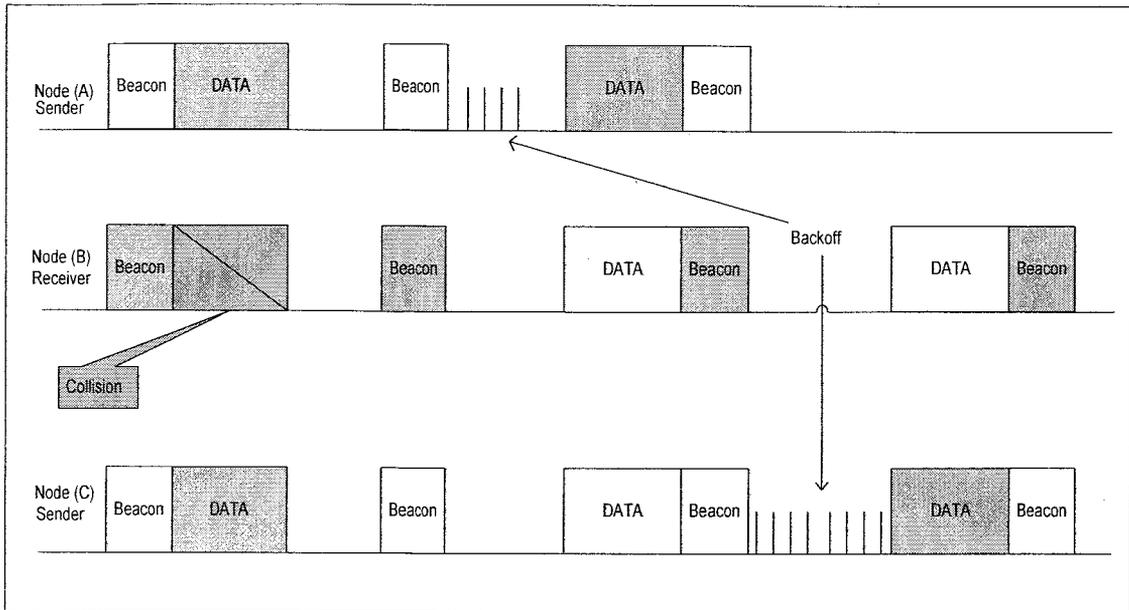
Figure 2.8 RI-MAC DATA frame transmission by back off mechanism [42]
