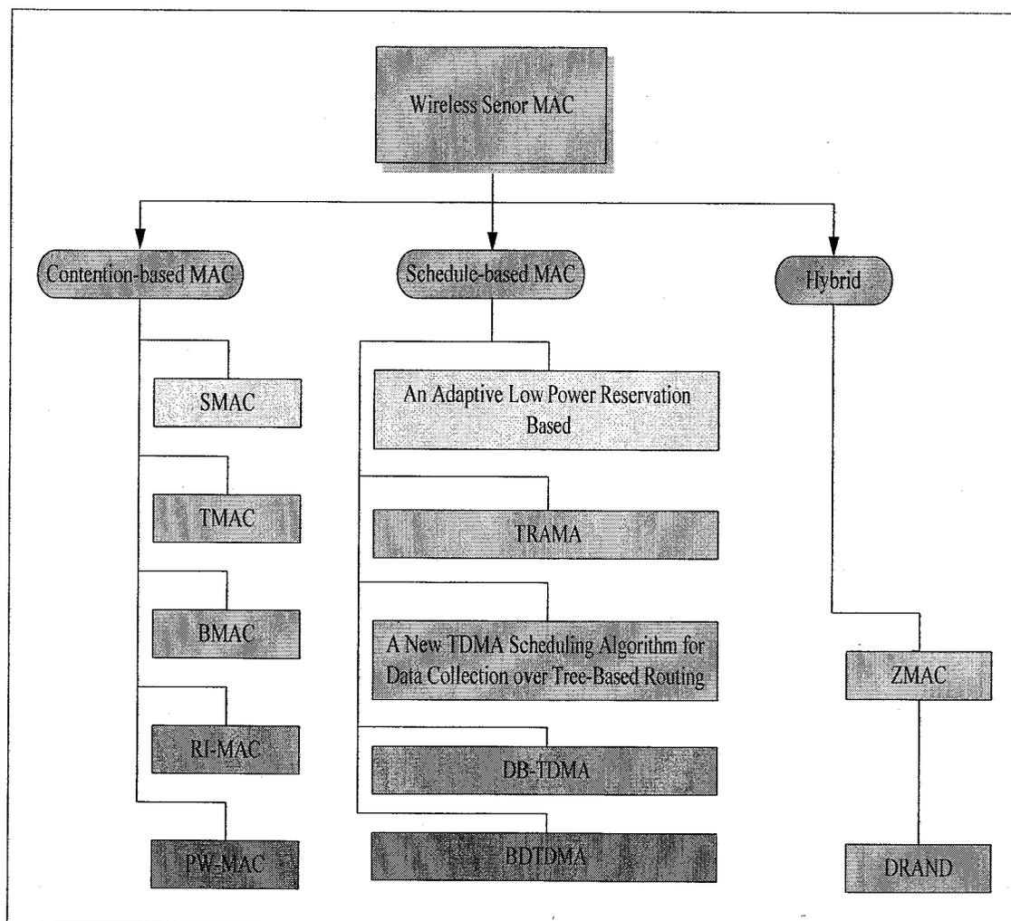
Figure 2.1 Categories and some examples of medium access control in WSNs
