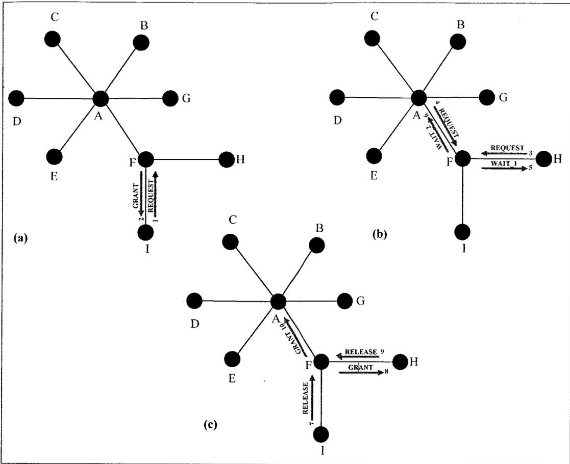
Figure 3.5 Slot assignments procedure in DSSA
