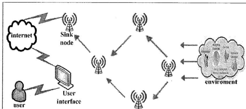
Figure 1.1 Data flow of WSNs from environment to end user
