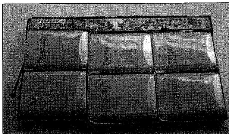
Figure 2.3: An inside look of the laptop battery [8]
