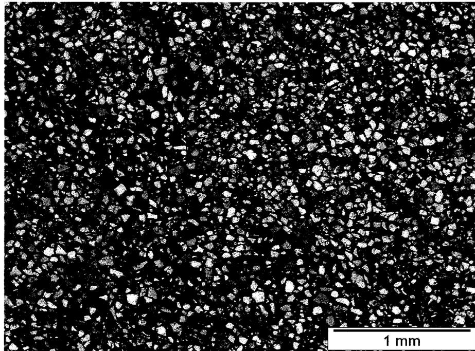
Figure 4.24: Sample NJ of Outcrop 2 under x4 magnification and plain polarize light.
