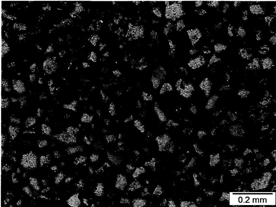
Figure 4.32: Sample JOC4 of Outcrop 4 under x10 magnification and plain polarize light.
