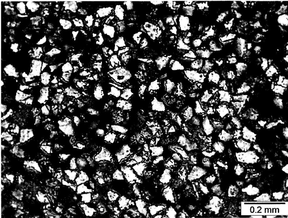
Figure 4.27: Sample NG1 of Outcrop 2 under x10 magnification and plain polarize light.
