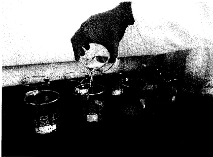
Figure 3.2: Pouring in the Hydroflouric Acid into the samples to remove the silica content.
