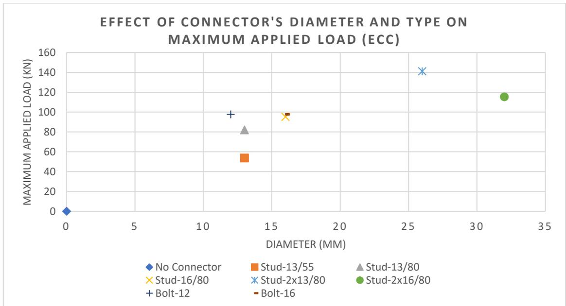
**Figure 4.6:** The effect of connector's diameter and type on maximum applied load (Engineered Cementitious Concrete).
