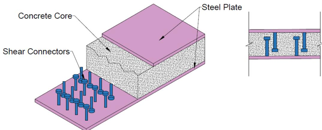
**Figure 1.1:** Steel-Concrete-Steel (SCS) sandwich structure with shear headed stud connectors.
