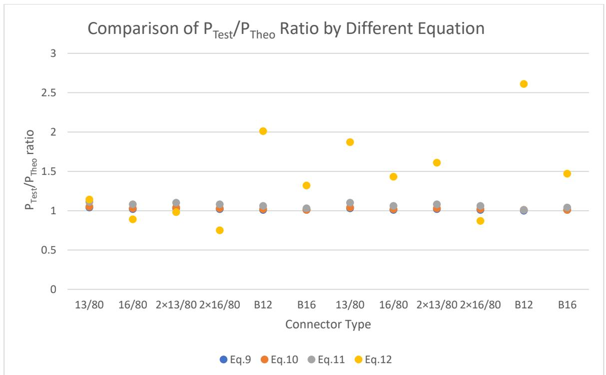
**Figure 4.4:** Comparison of  $P_{Test}/P_{Theo}$  Ratio by Different Equation.
