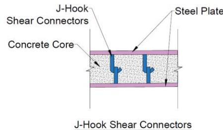
**Figure 2.3:** SCS sandwich with J-Hook shear connectors.
