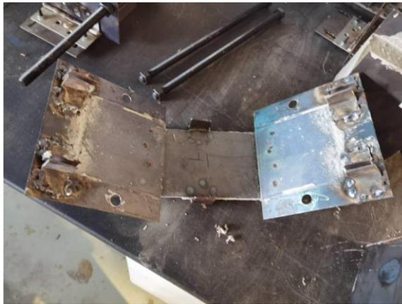
**Figure 3.1:** Steel formwork for specimen preparation.
