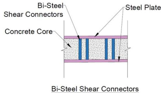
**Figure 2.2:** SCS sandwich with Bi-Steel shear connectors.
