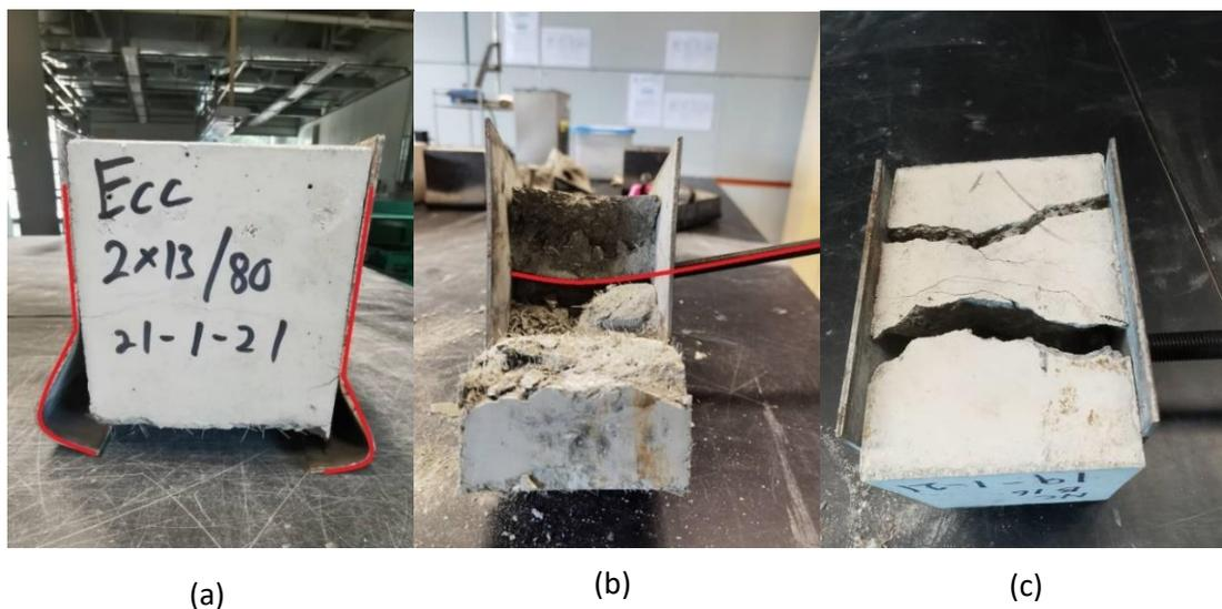
**Figure 4.1:** (a) Steel buckling. (b) Bolt bending. (c) Concrete crushing and cracking.
