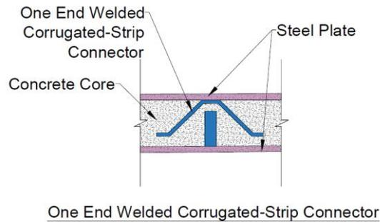
**Figure 2.5:** SCS sandwich with One End Welded Corrugated-Strip shear connectors.
