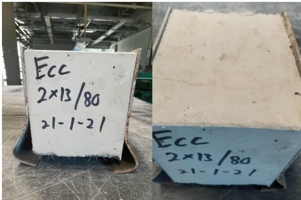
**Figure 4.7:** Steel plate buckling with minor crack.
