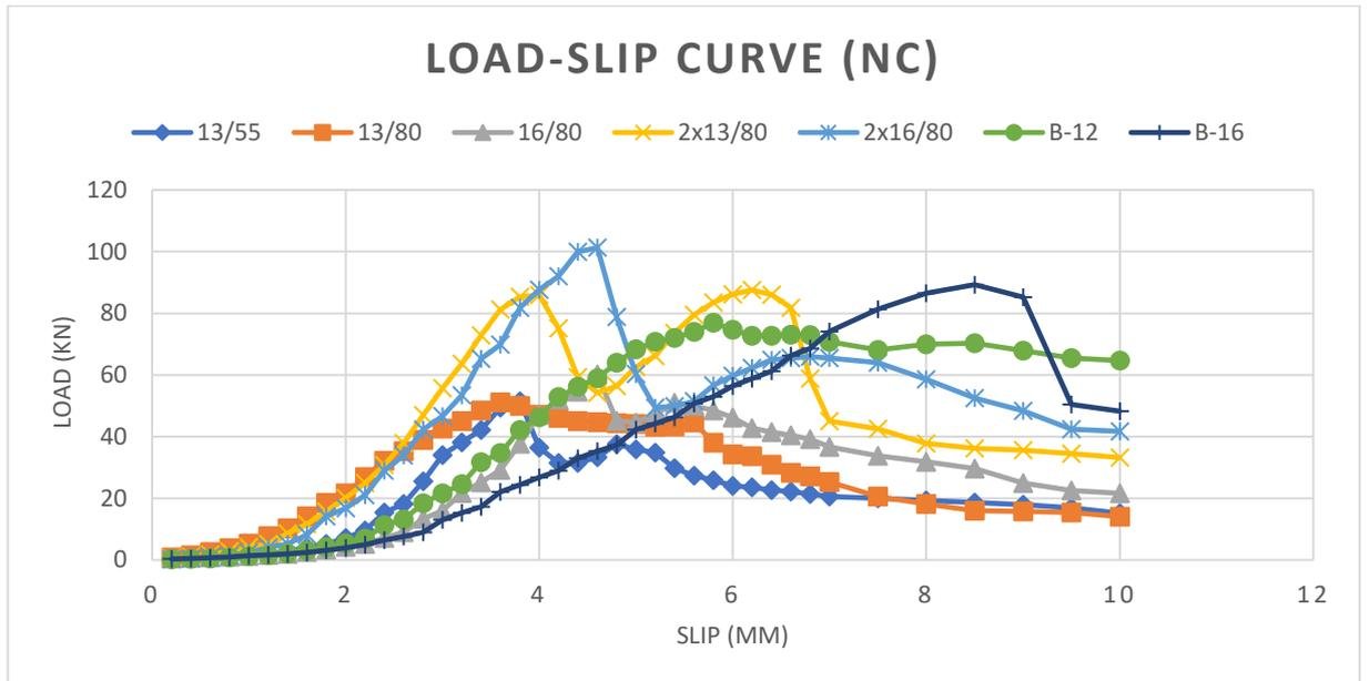
**Figure 4.2:** Load-Slip Curve (NC).
