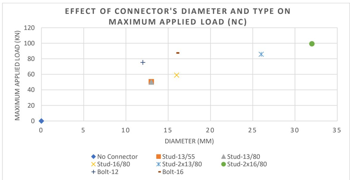
Figure 4.5: The effect of connector's diameter and type on maximum applied load (Normal Concrete).
