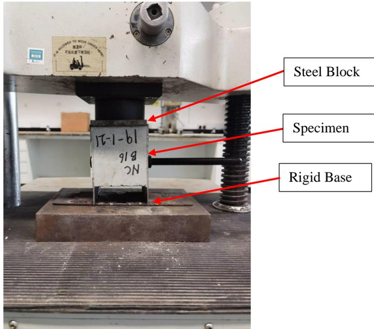
**Figure 3.2:** Test setup.
