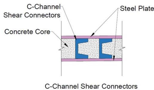
**Figure 2.4:** SCS sandwich with C-Channel shear connectors.
