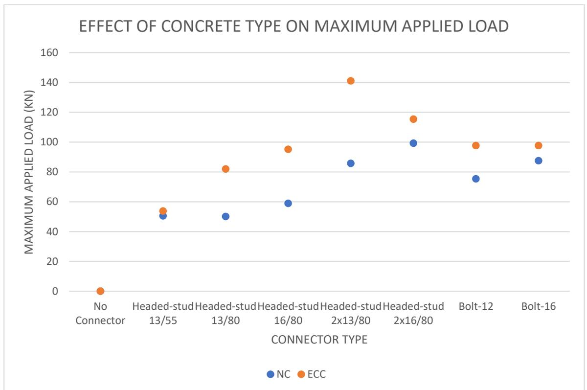
**Figure 4.8:** Effect of concrete type on maximum applied load.
