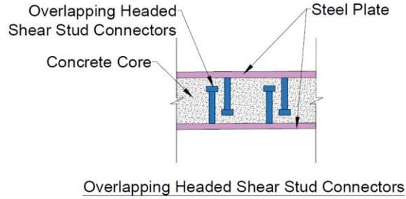
**Figure 2.1:** SCS sandwich with overlapping headed stud shear connectors.
