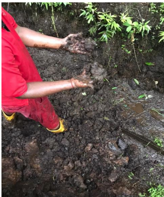
Figure 3.3: Von Post Humification Test Conducted on Site
