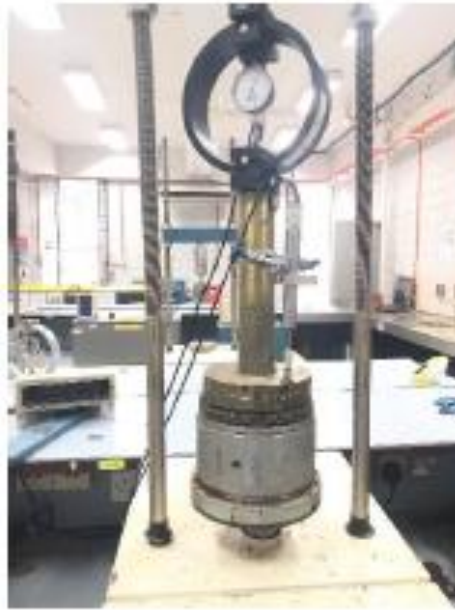
Figure 3.8: California bearing ratio (CBR) Testing Machine
