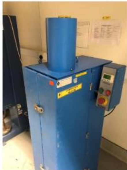
Figure 3.6: Standard Proctor Compaction Machine
