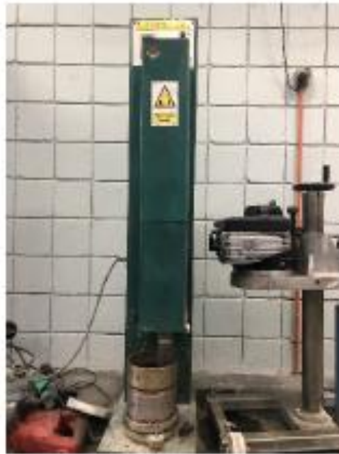
Figure 3.9: California bearing ratio (CBR) Testing Compaction Machine
