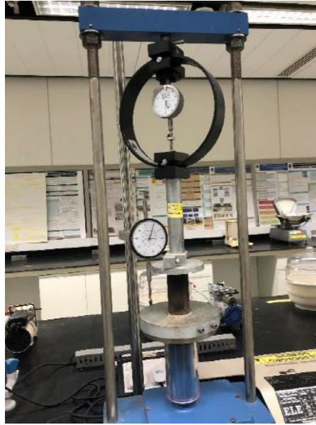
Figure 3.7: Unconfined Compression Strength (UCS) Test
