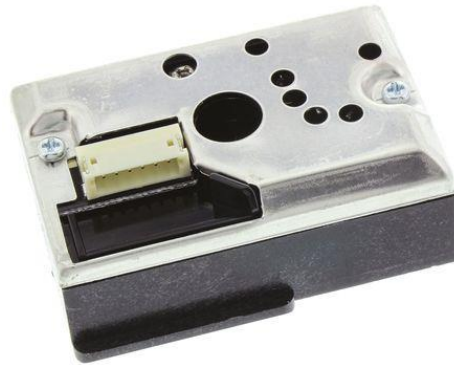
Figure 10. SHARP GP2Y1010AU0F PM 10 Sensor [24]
