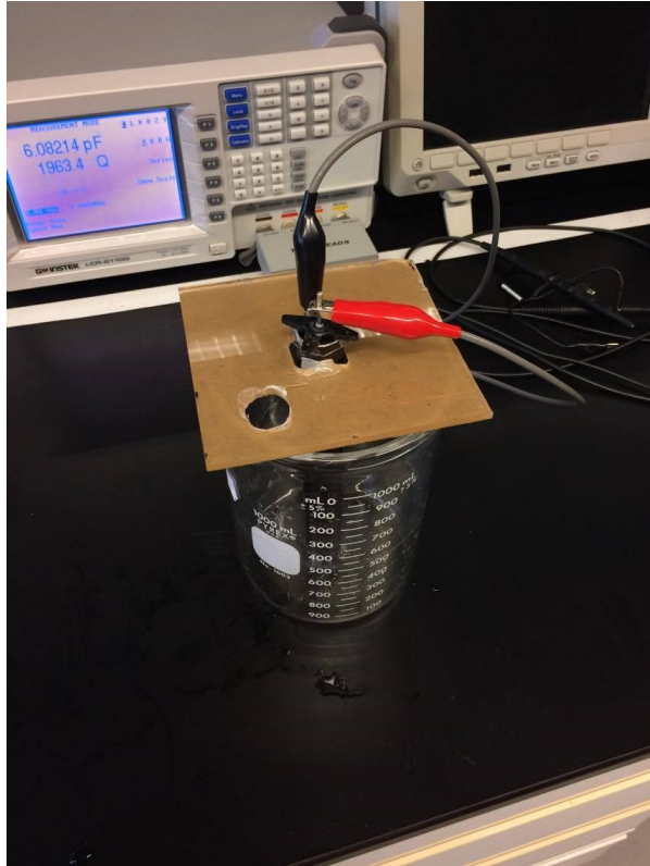
Figure 22 setup for capacitance based liquid sensor experiment
