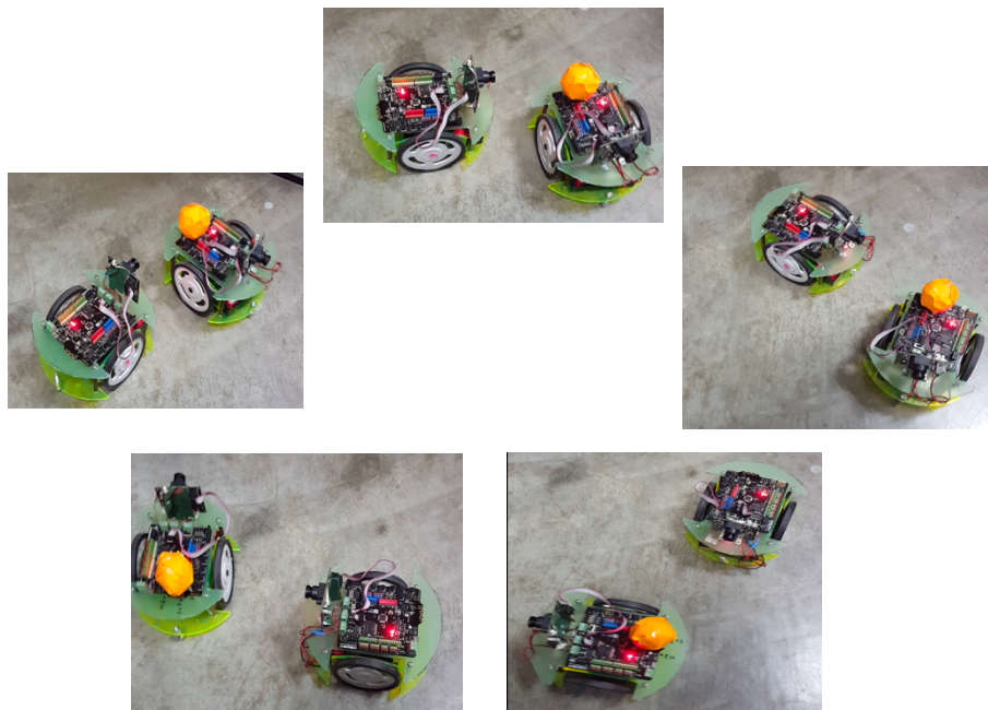
Figure 17: Platooning trajectory when moving in circle
