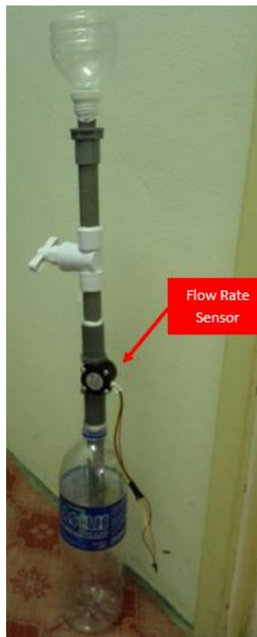
Figure 13. Testing on the Flow Rate Sensor
