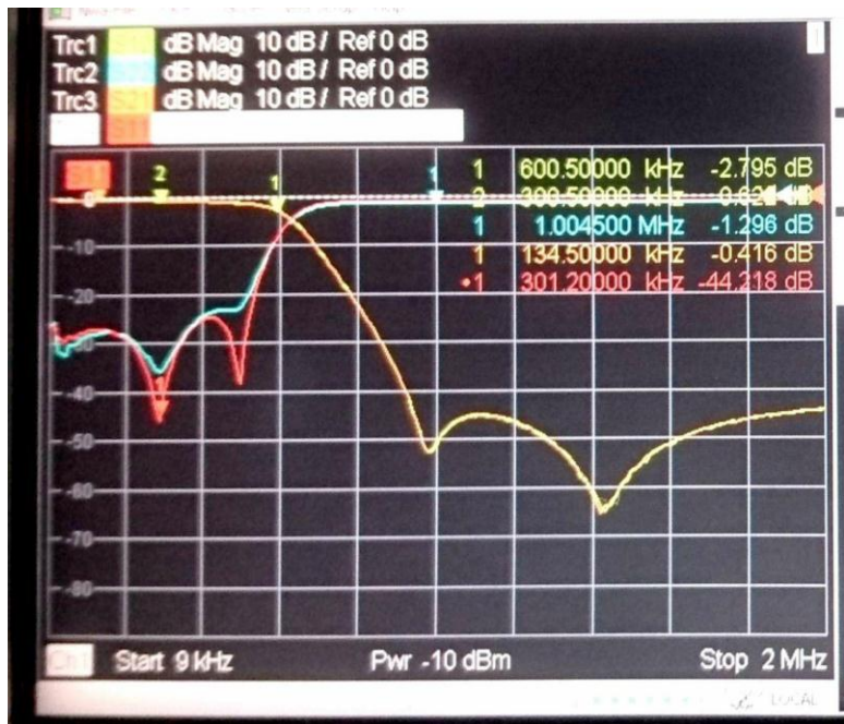
Figure 47 : Frequency vs Attenuation response recorded using data obtained from the Inverse Chebyshev experiment.
