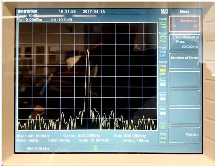
Figure 50 : FFT waveform measured at the output of Inverse Chebyshev filter
