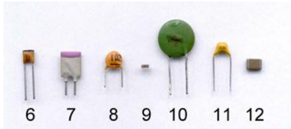
Fig #: Ceramic capacitors, low 'k', 33pF (6), medium 'k', 330pF - 1.5nF (7, 8, 9), high 'k', 100nF (10, 11, 12)
