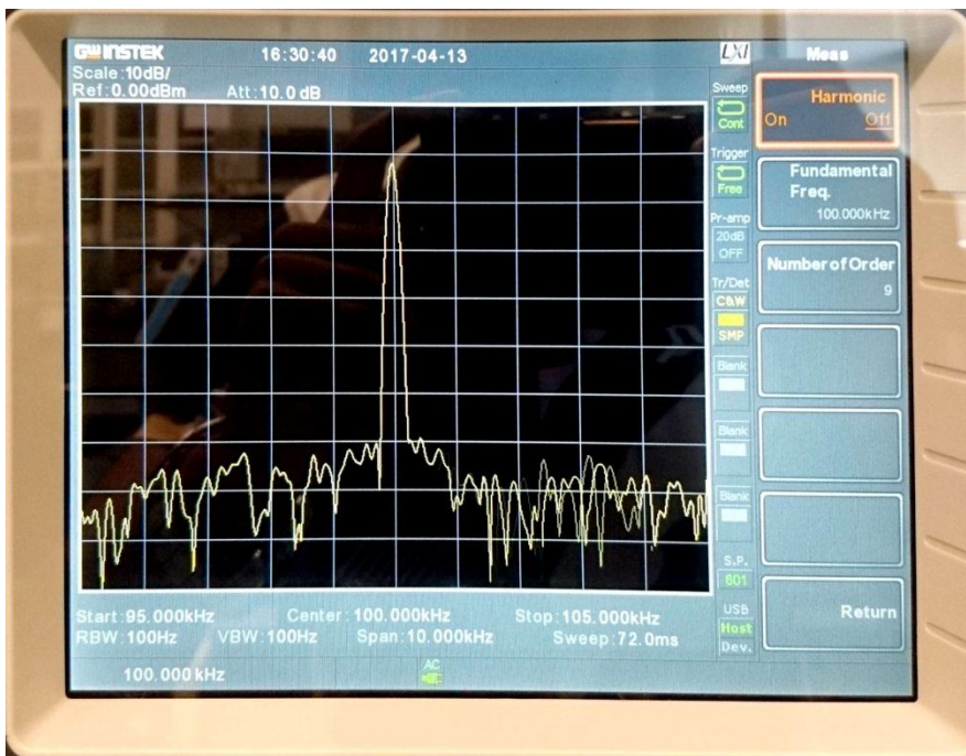
Figure 42 : FFT waveform measured at the output of Chebyshev filter
