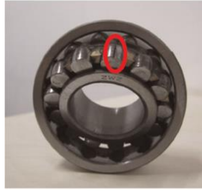
Figure 2: Roller element defects
