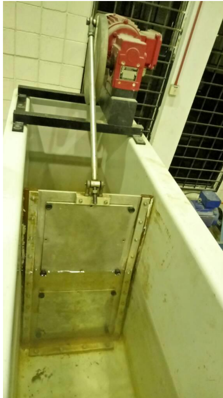
FIGURE 3.2 Wave Generator inside wave flume.
