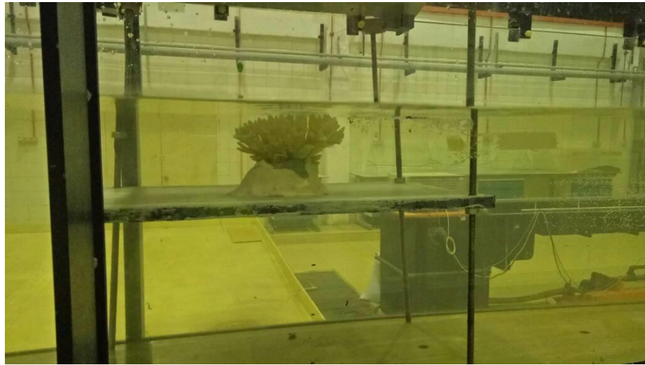
FIGURE 3.4 Acropora Millepora sp. coral fixed on adjustable plywood stand.
