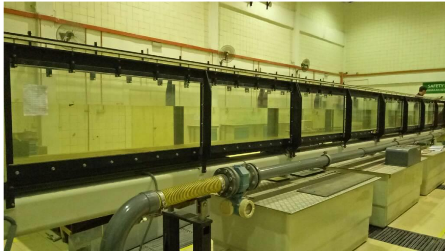
FIGURE 3.1 Wave flume used for experimental process.
