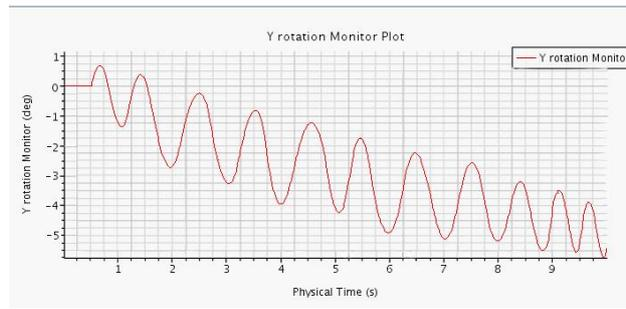
**Figure 4. 4 Numerical Expected Yaw Motion with rotating fan blade**
