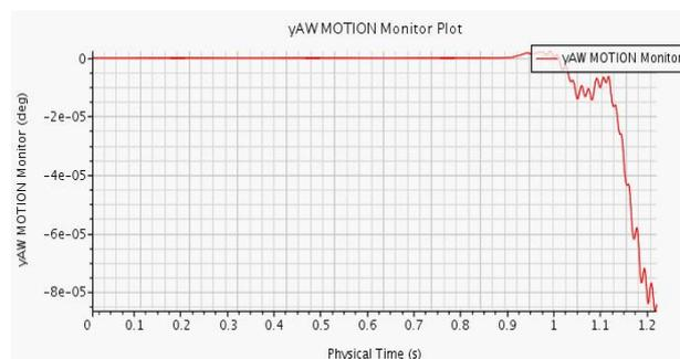
**Figure 4. 3 Numerical Yaw Motion with rotating fan blade**
