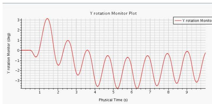
**Figure 4. 2 Numerical Expected Yaw Motion with no rotating fan blade**
