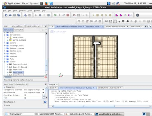
Figure 3. 3 The volume meshing of the environment
