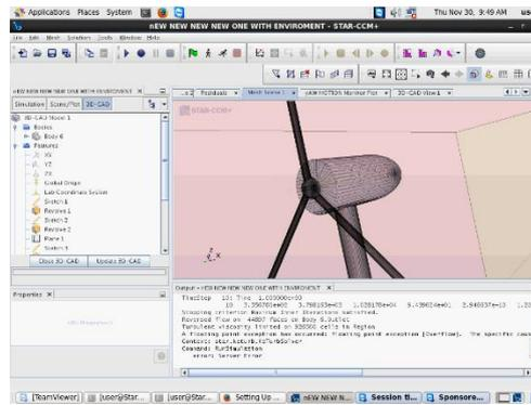
Figure 3. 2 The surface meshing on the FOWT
