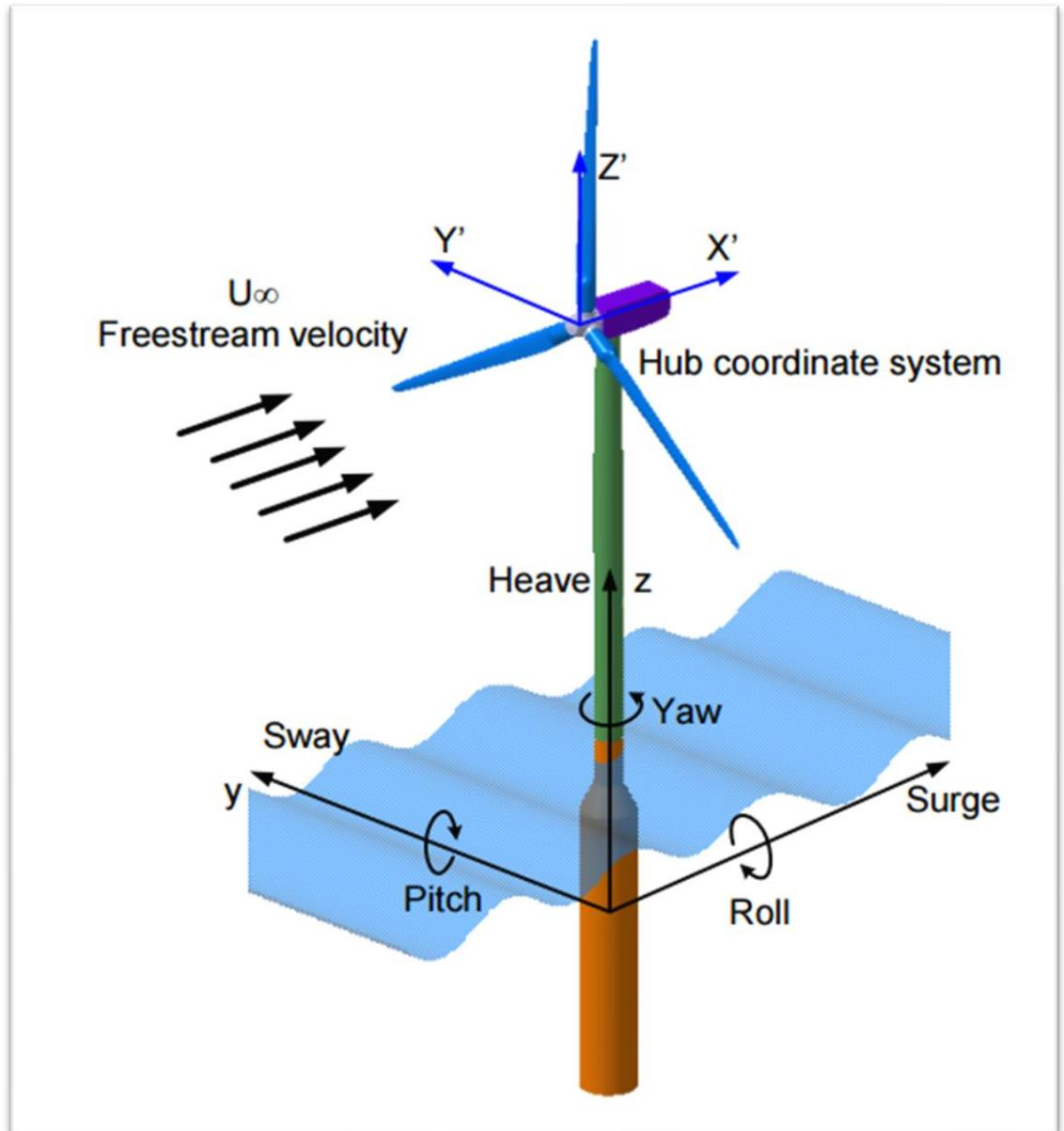
Figure 2. 1 Resultant motion produce in FOWT
