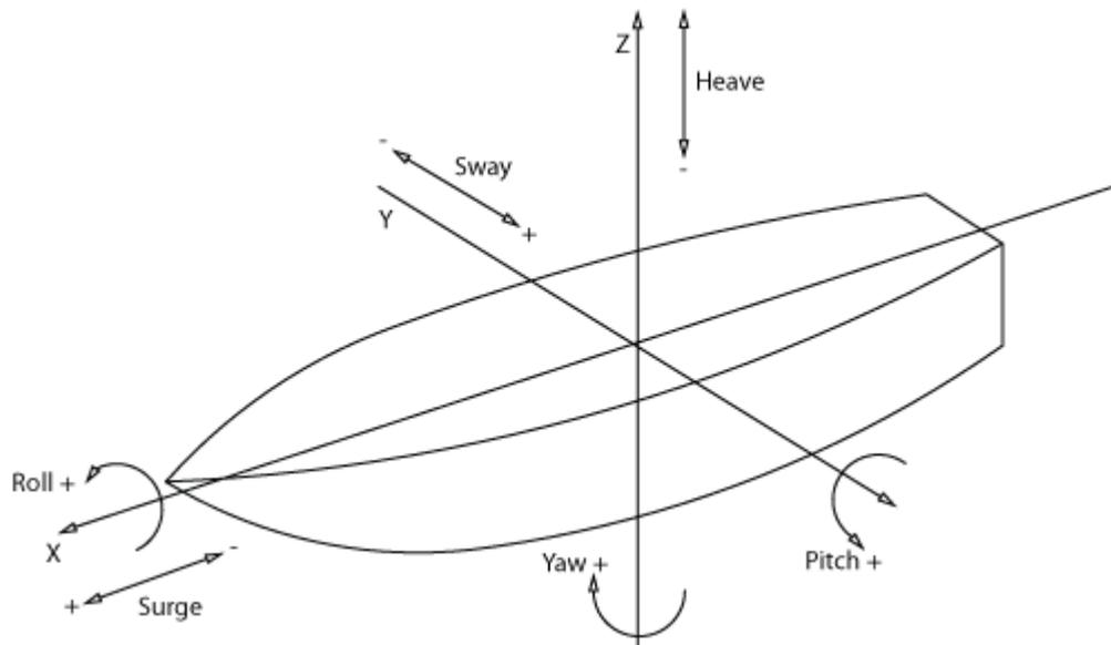
Figure 1. 1 Reaction of floating structure upon load acting on them.
