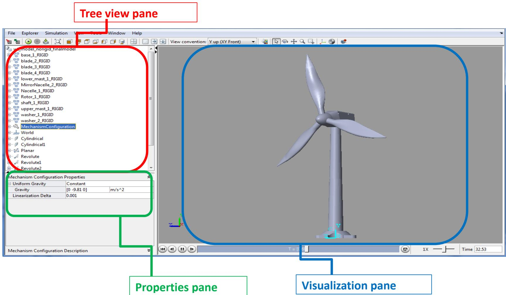
Figure 20: Visualization of Wind Turbine Model in Mechanics Explorer during Simulation
