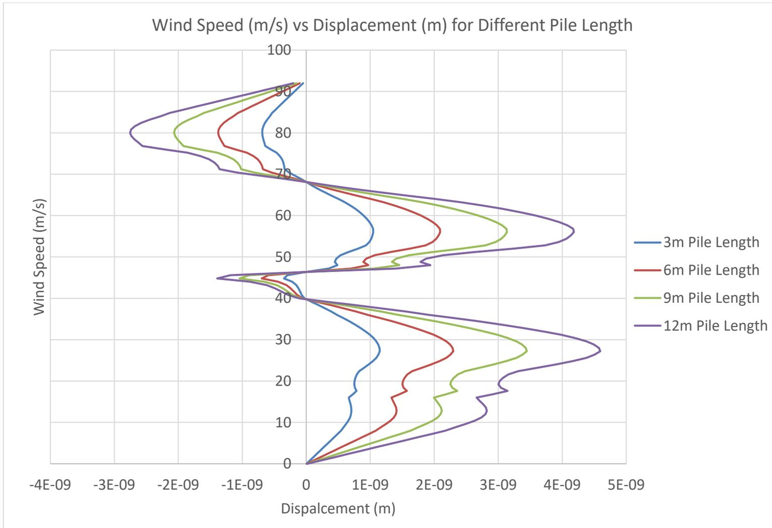
**Figure 29: Wind Speed vs. Displacement for Different Pile Length**
