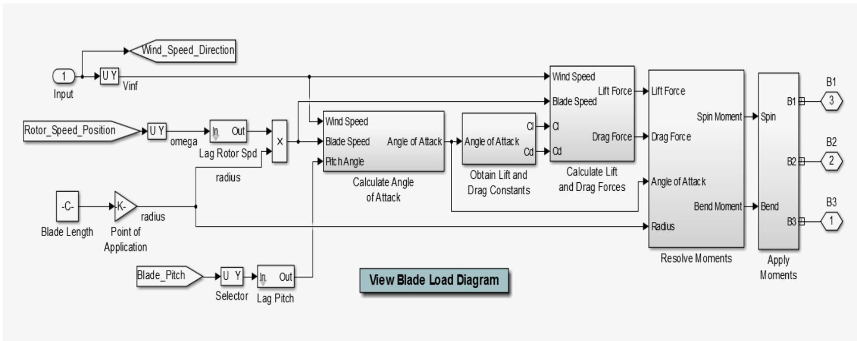
Figure 16: Blade Load Model
