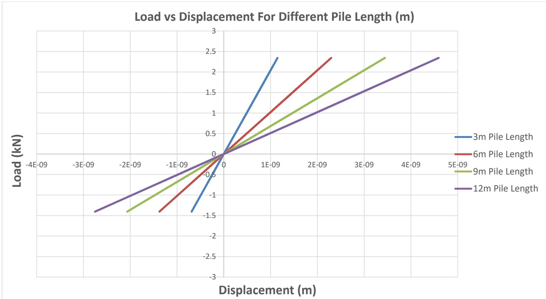
**Figure 27: Load vs. Displacement for Different Pile Length**
