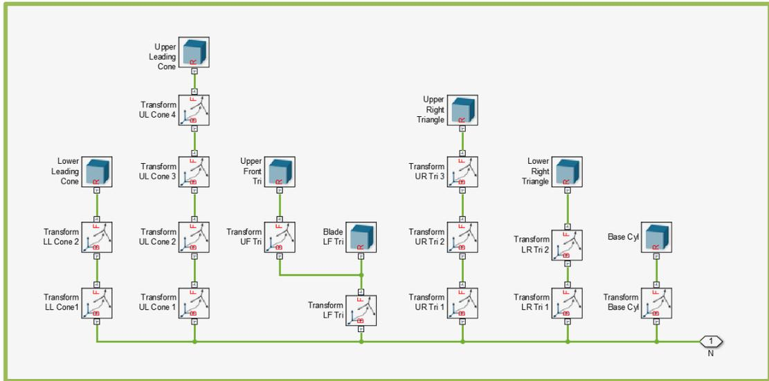
**Figure 13: Elements of Blade Model**
