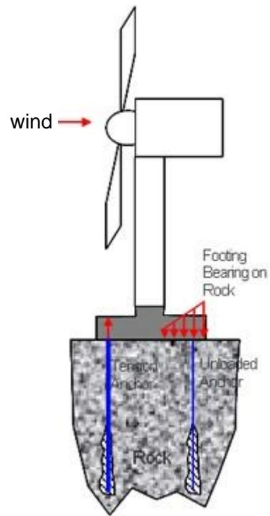
**Figure 6: Anchored Footing**
