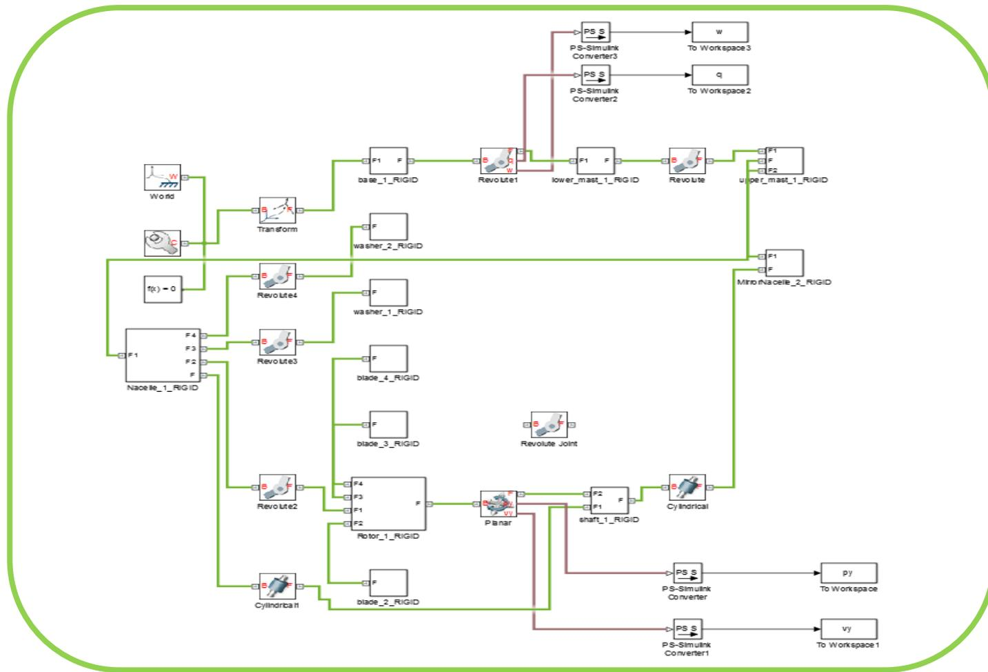
Figure 19: Physical Model of Wind Turbine in Simmechanics Blocks
