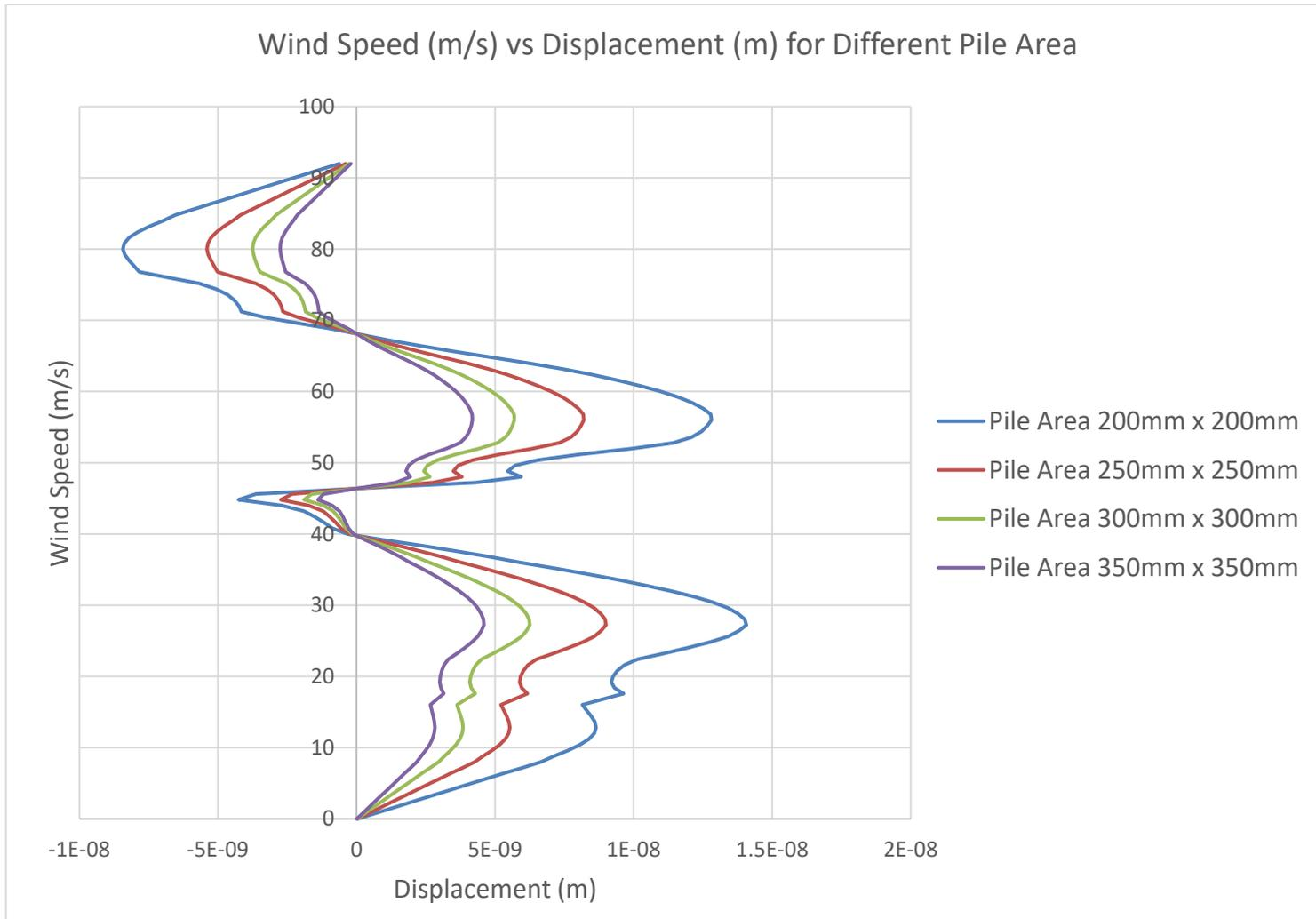
**Figure 30: Wind Speed vs. Displacement for Different Area of Pile**
