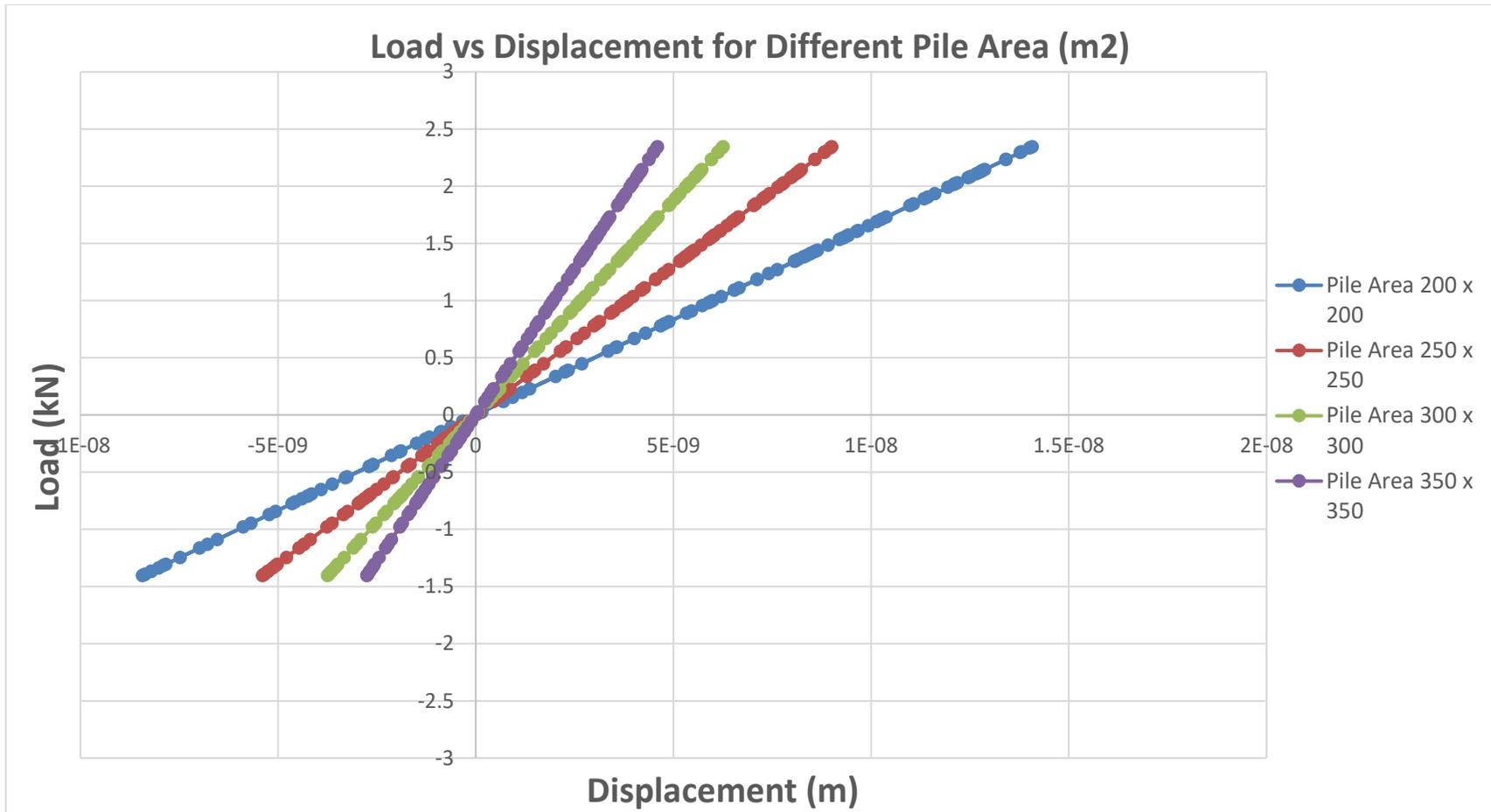
**Figure 28: Load vs. Displacement for Different Area of Pile**
