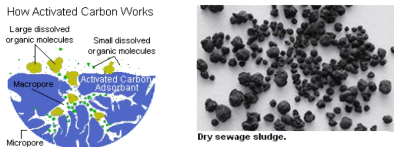
FIGURE 2 : How Activated Carbon Works & Samples of Dry Sewage Sludge
