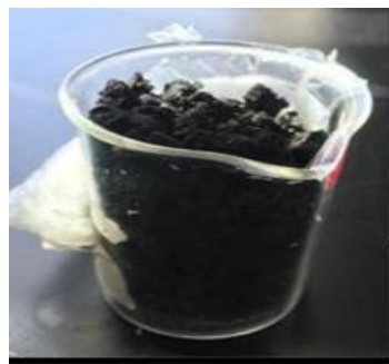
FIGURE 6: Initial dried sludge directly carbonized by pyrolysis at 500 °C
