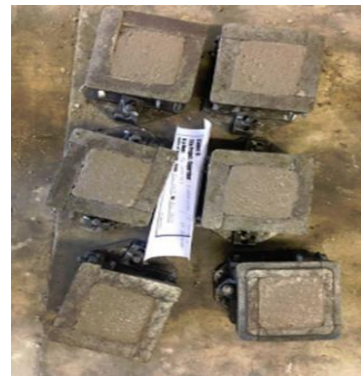
Figure 3.3 Concrete mix in mould
