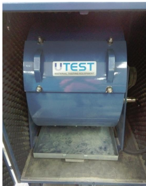
Figure 3.12 Los Angeles abrasion machine
