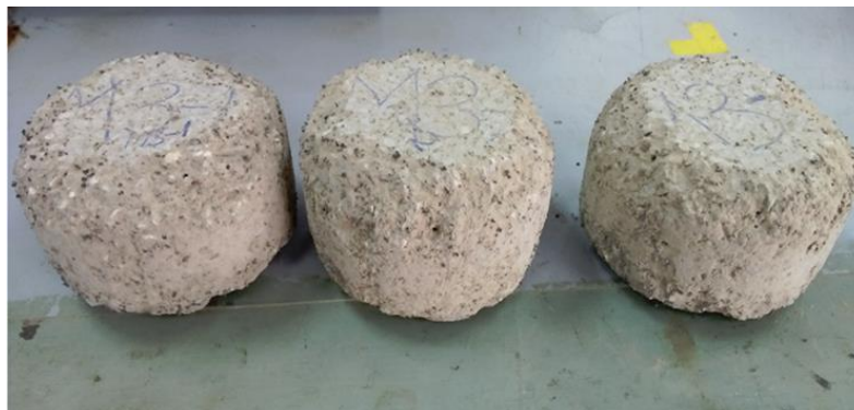
Figure 3.16 Shape of specimen after abrasion test for 300 revolutions
