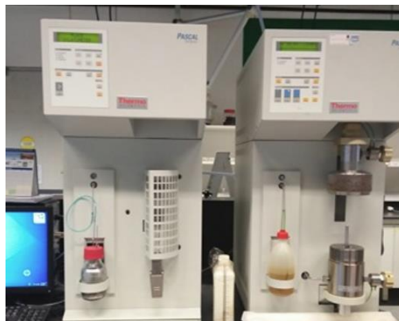
Figure 3.17 Mercury Intrusion Porosimeter machine
