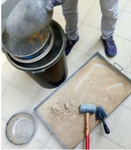
Figure 3.2: Top Soil is Crushed and Sieved Using 2mm Sieve Size
