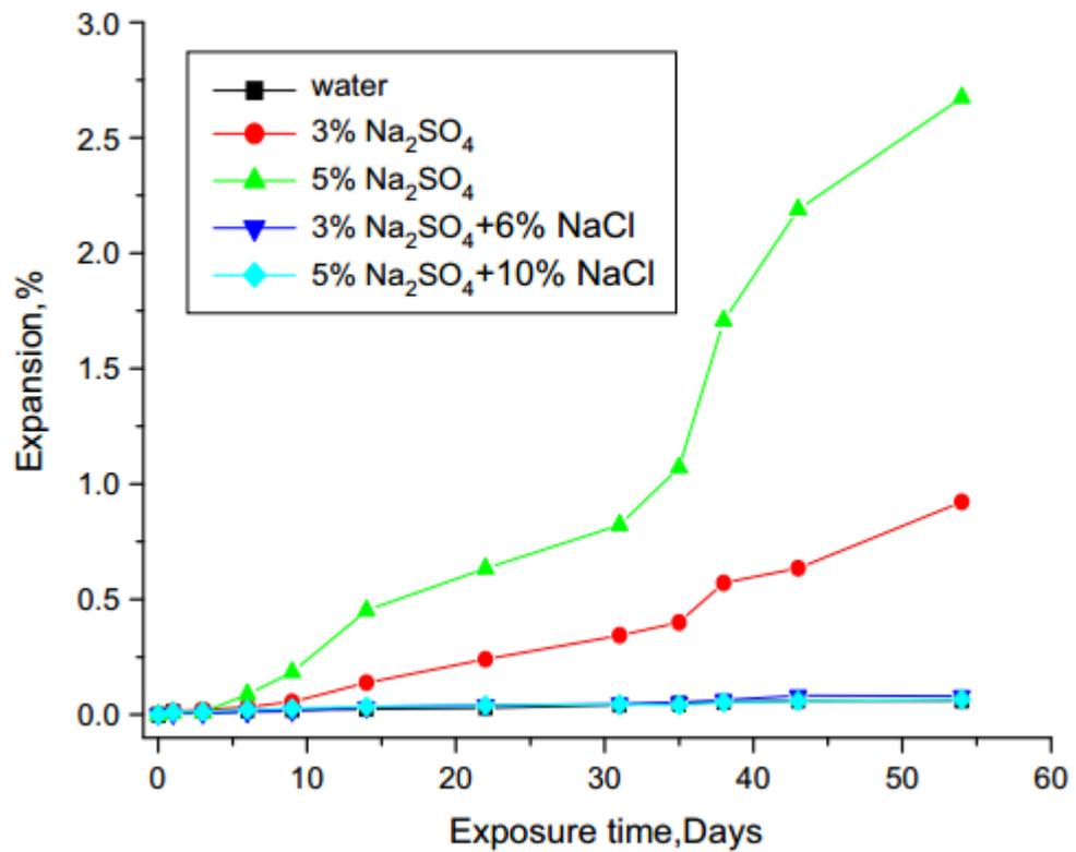
Figure 4. 11 Axial Expansion of Samples Being Immersed in Different Solutions
