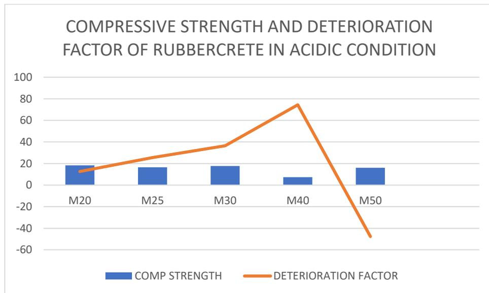
Figure 4. 9 Compressive Strength And Deterioration Factor in Acid Condition
