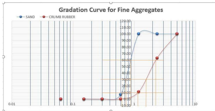
Figure 4. 1 Gradation Curve for Fine Aggregate
