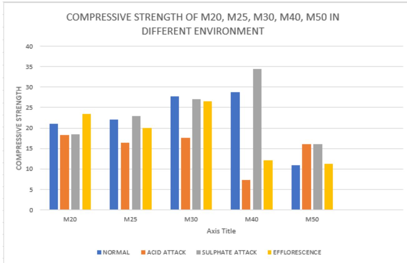
Figure 4. 8 Compressive Strength of M20, M25, M30, M40 and M50 in Different Exposure
