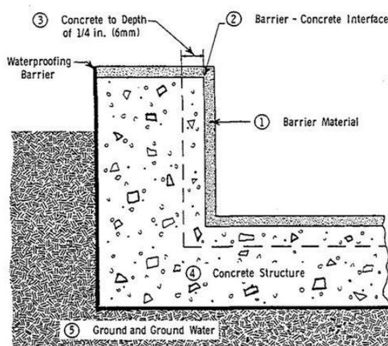
Figure 2. 1 - Chemical Attack Precautions In Concrete Structure (Types of Chemical Attacks on Concrete Structure, 2017)
