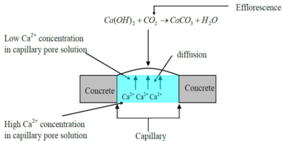
Figure 2. 2 - Schematic diagram of efflorescence from cross sectional view of concrete block
