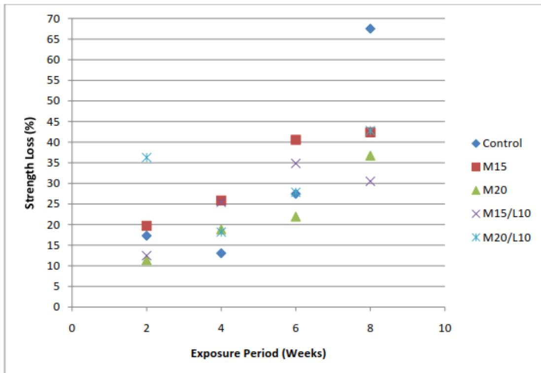
Figure 4. 10 Strength Loss of Concrete Samples after Exposure to a 5% Sulphuric Acid Solution
