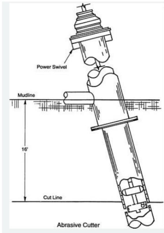
FIGURE 3 SCHEMATIC OF A MECHANICAL CUTTING SYSTEM (SNYDER & BYRD, 2004)
