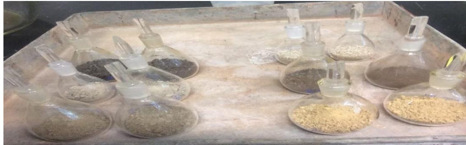
FIGURE 3. 2 Small Pycnometer Method for Specific Gravity Experiment
