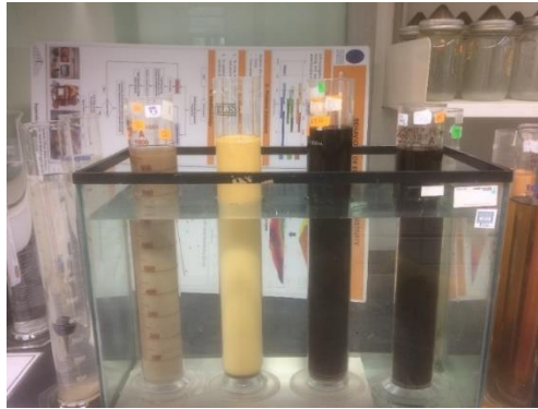
FIGURE 3. 5 Hydrometer Test for Particle Size Distributions
