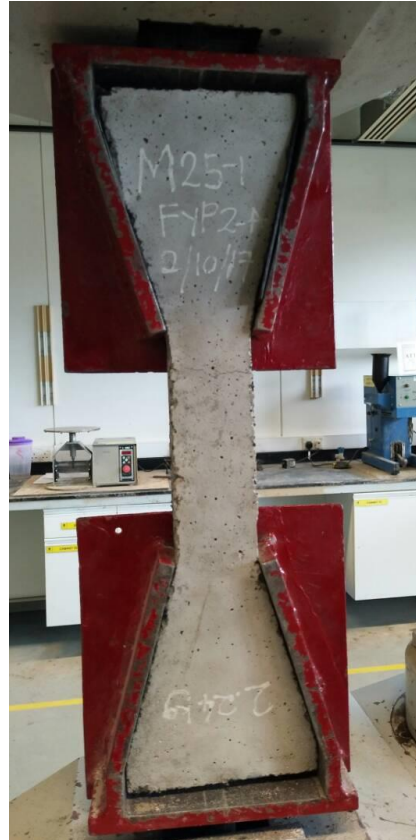
Figure 4.3: Direct Tensile Test Configuration
