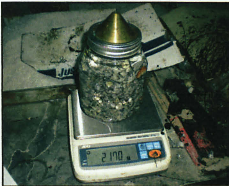
Figure 13: Weighing the aggregate during the specific gravity test
