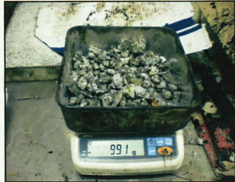
Figure 13: Weighing the aggregate during the specific gravity test
