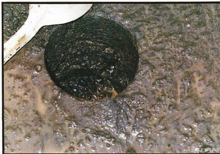
Figure 3: Small pavement core showing stripping at the bottom of the pavement section
