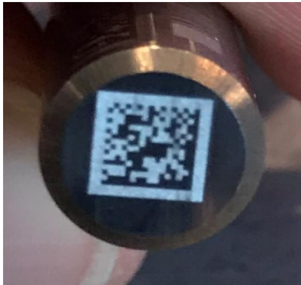
Figure 6. Data Matrix code engraved on a drill bit
