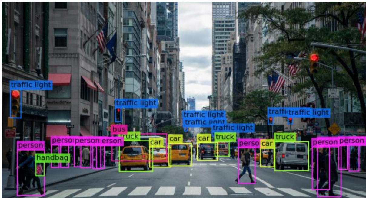
Figure 2.7.1 Example of Computer Vision with Object Detection
