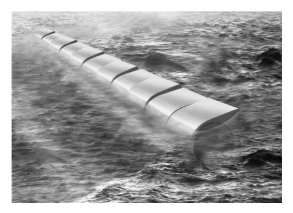
FIGURE 2.6: Salter's Nodding Duck wave energy converter.
