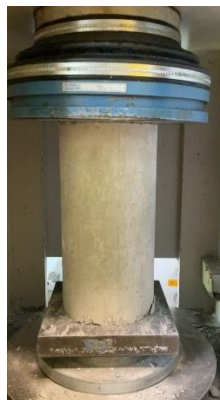
FIGURE 3.6: Compression Machine and Specimen Before Testing.
