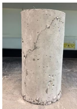
FIGURE 4.5: Failure Mode of Specimen
