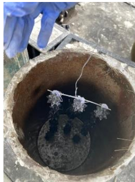
FIGURE 3.5: Position of Origami Hollow Aggregate during Casting
