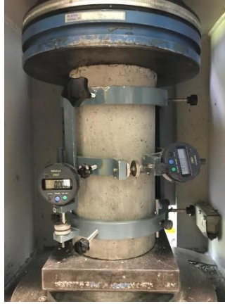
FIGURE 3.7: Compressometer-Extensometer for Modulus of Elasticity Test
