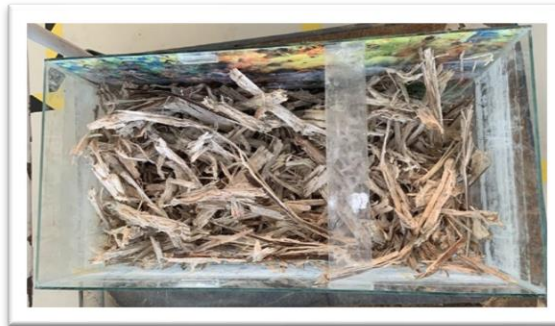
FIGURE 3.3. SCB in 0.1 M HCl solution
