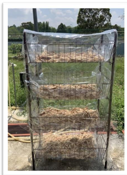
FIGURE 3.4. Pre-Treated SCB in drying chamber
