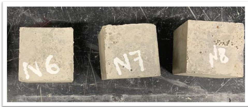
FIGURE 4.6. Untreated concrete sample (Left to Right: 600°C, 700°C and 800°C)
