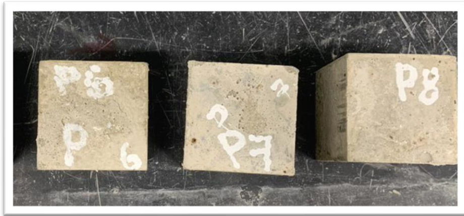
FIGURE 4.5. Pre-treated concrete sample (Left to Right: 600°C, 700°C and 800°C)
