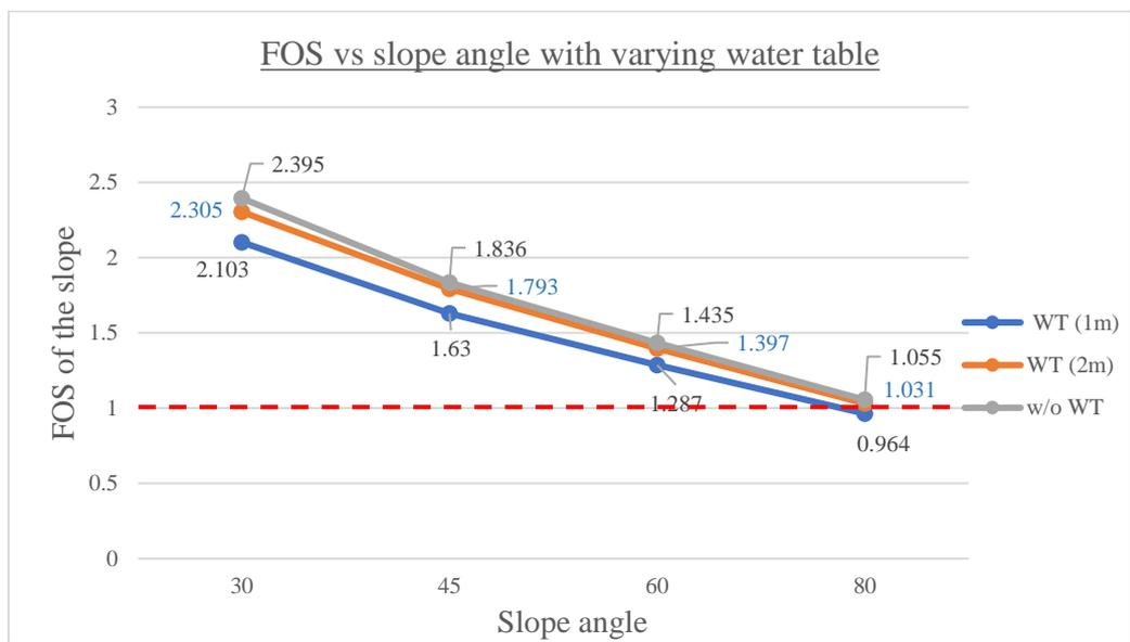
FIGURE 4.2.2 Factor of safety vs the slope angle for set 2 (b)
