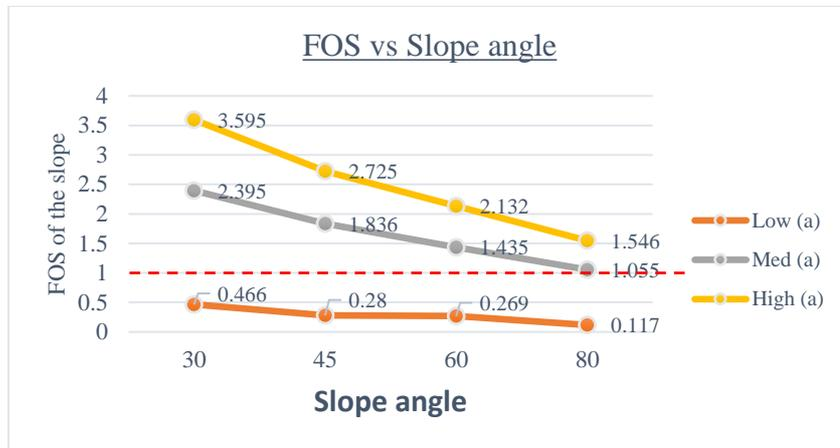
FIGURE 4.1.3 Factor of safety vs the slope angle for set 1 (a)
