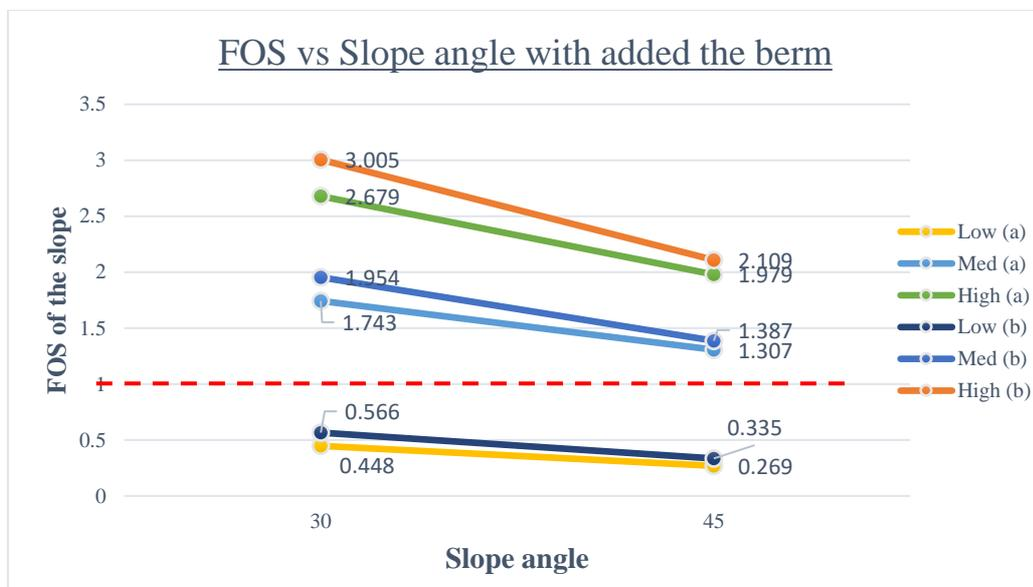
FIGURE 4.2.8 Factor of safety vs the slope angle for 6m slope height
