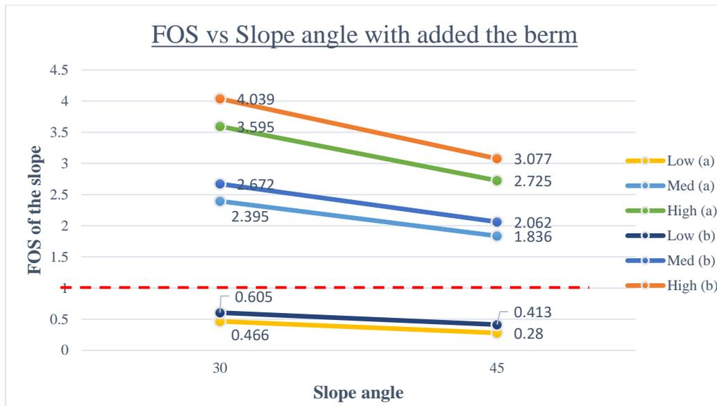
FIGURE 4.2.7 Factor of safety vs the slope angle for 3m slope height
