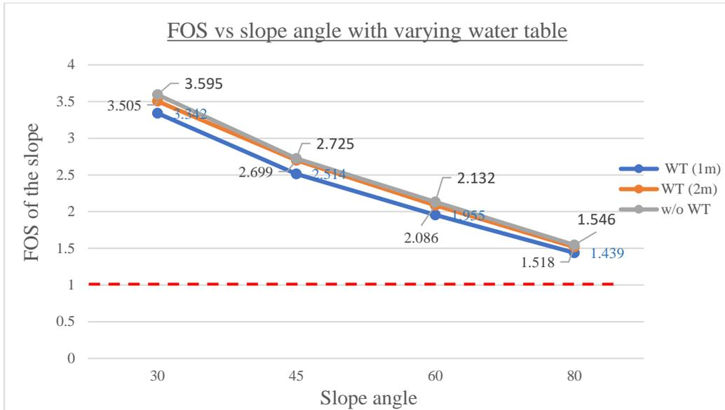
FIGURE 4.2.3 Factor of safety vs the slope angle for set 2 (c)
