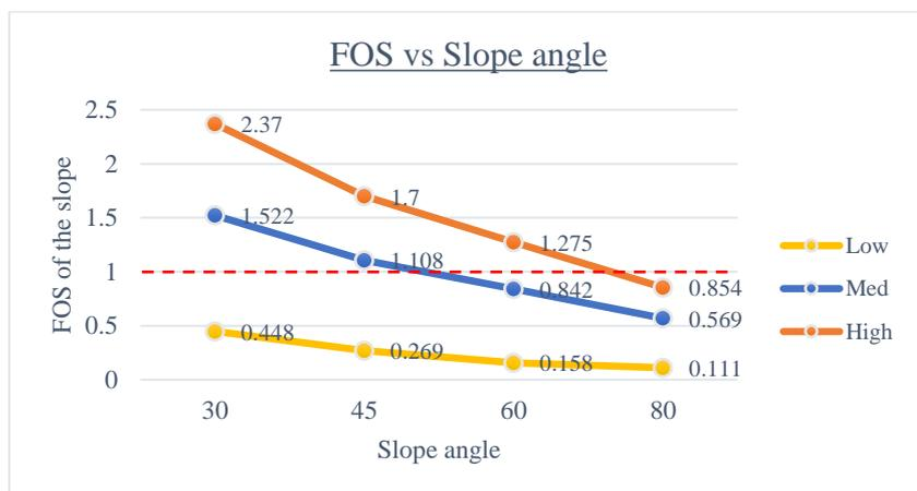
FIGURE 4.1.3 Factor of safety vs the slope angle for set 1 (c)
