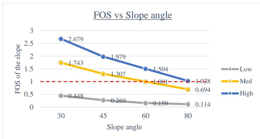
FIGURE 4.1.2 Factor of safety vs the slope angle for set 1 (b)
