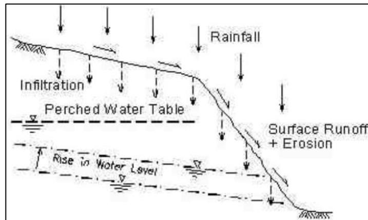
FIGURE 2.3.1 Effects of rainfall on high permeable slope
