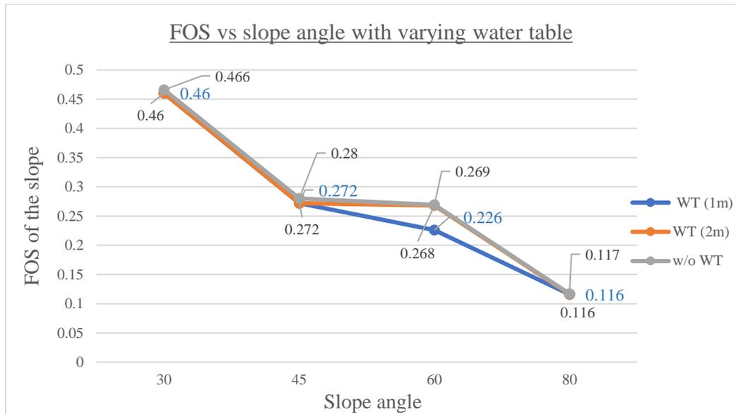
FIGURE 4.2.4 Factor of safety vs the slope angle for set 2 (a)
