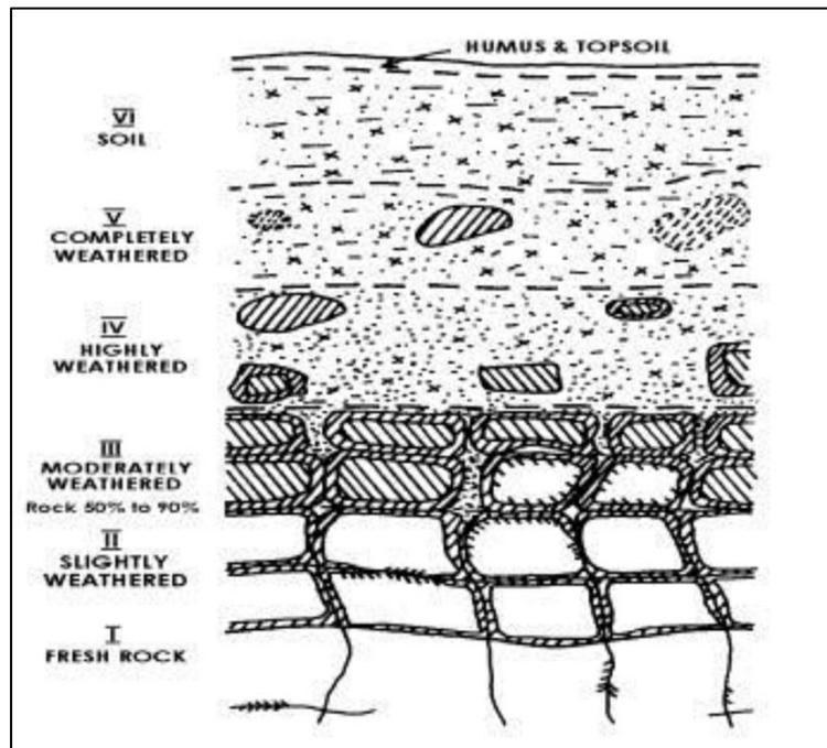
FIGURE 2.2 Typical weathering profile of residual soil
