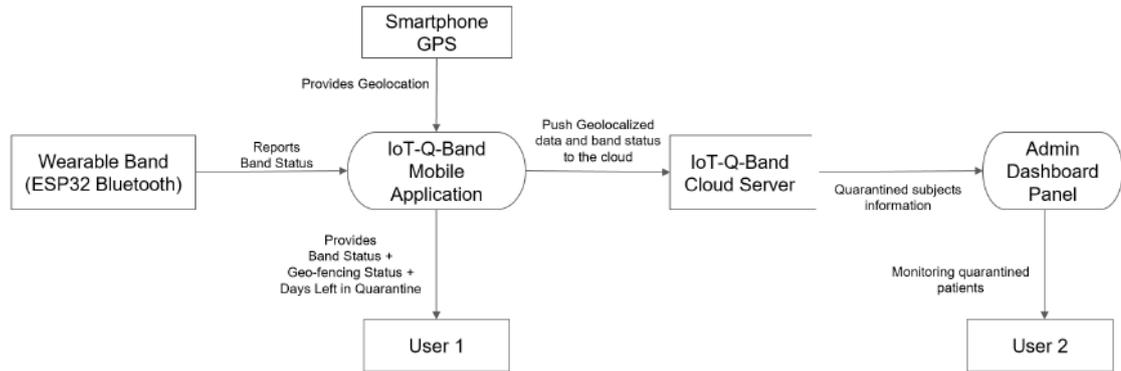
Figure 2 : IoT Q-Band Dataflow
