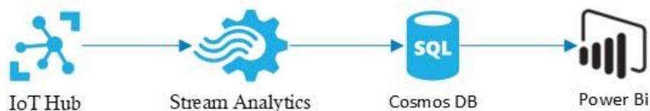
Figure 16: Back-End System Flow
