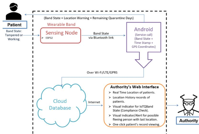
Figure 1 : IoT Q-Band System Architecture
