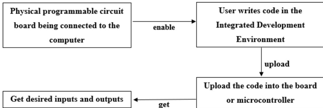
Figure 4: Arduino Development Process
