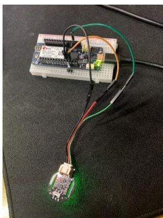
Figure 33: Heartrate Sensor Connected
