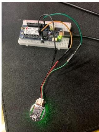
Figure 33: Heartrate Sensor Connected
