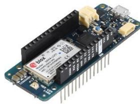
Figure 17: Arduino MKR GSM 1400
