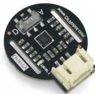
Figure 19: DFRobot Heartrate Sensor
