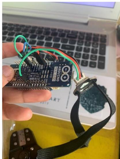
Figure 22: Connection of Heartrate Sensor
