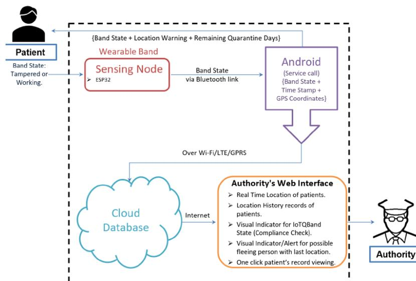
Figure 1 : IoT Q-Band System Architecture
