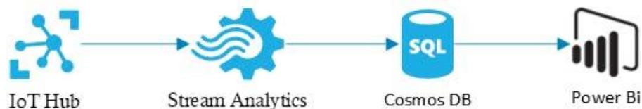
Figure 16: Back-End System Flow
