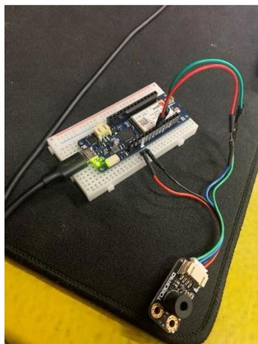
Figure 30: Temperature Sensor Connected
