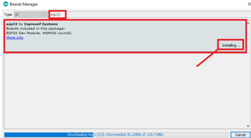
Figure 4.5: Interface of ESP32 installation.
