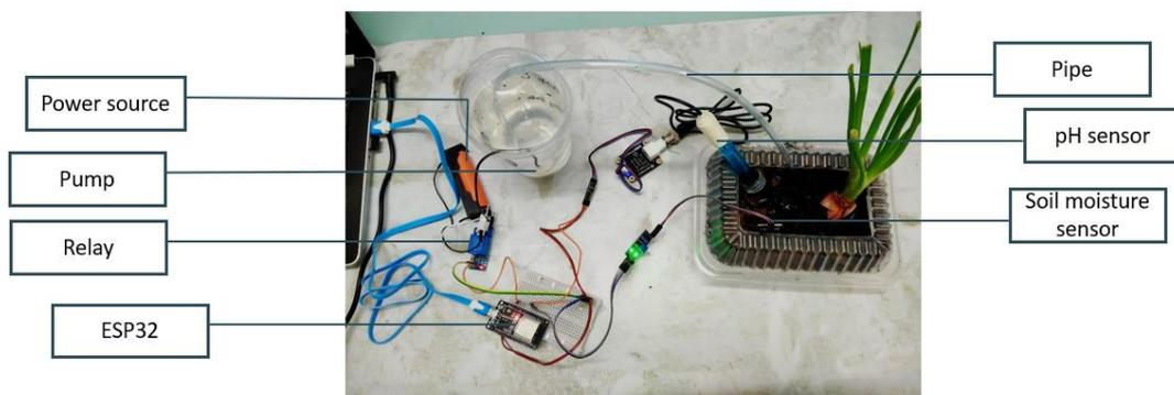
Figure 3.9: Hardware setup.
