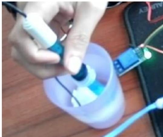
Figure 4.16: Place the pH meter sensor into the water.
