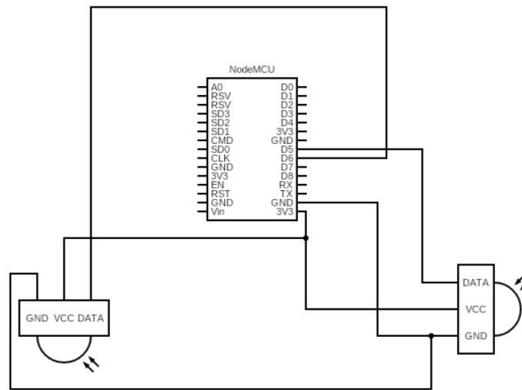
Figure 3.8: Circuit of an automated water sprinkler.
