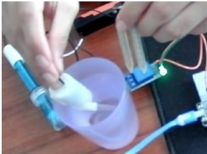
Figure 4.11: Place the soil moisture sensor out of the water.
