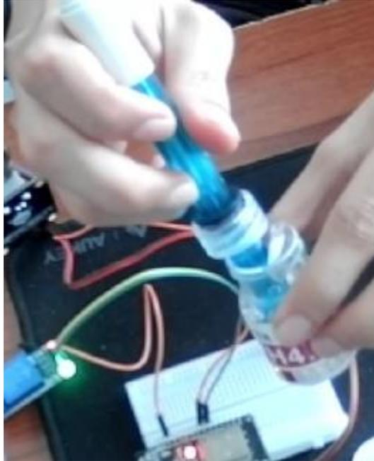
Figure 4.18: Place the pH meter sensor into buffer solution.
