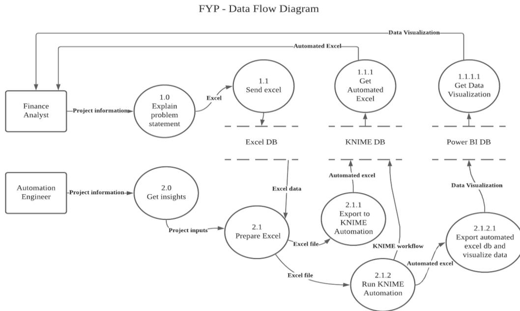
Figure 17 Data Flow Diagram
