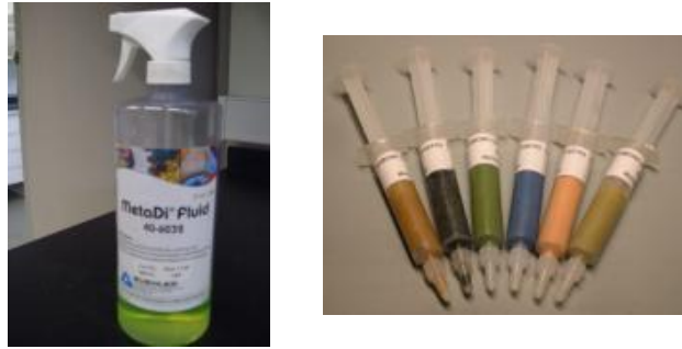
Figure 3.7: metaDi Fluid (Left) and Diamond Paste (Right).
