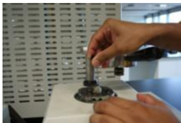
Figure 3.4a: The mounting is cleaned using release agent.
