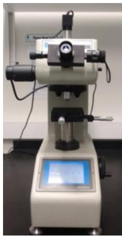
Figure 3.10: Microhardness Testing Machine used for indentation test.
