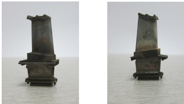
Figure 1.1: Turbine blade 1 st stage.
