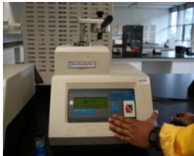
Figure 3.3: Equipment used for hot mounting.
