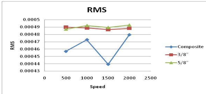
Figure 4.12: RMS versus speed at accelerometer 2.
