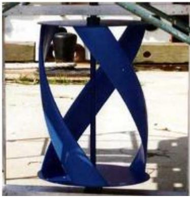
Figure 6: Gorlov Helical Turbine
