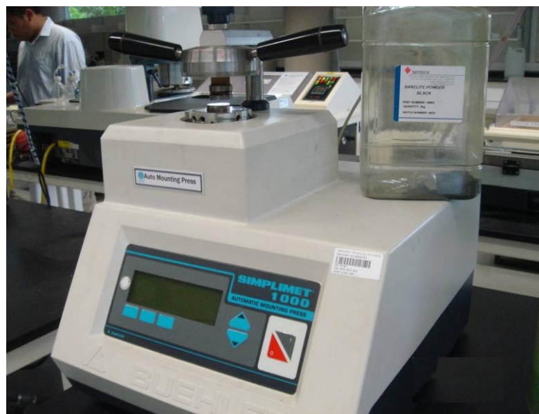
Figure 8 : Automatic mounting machine
