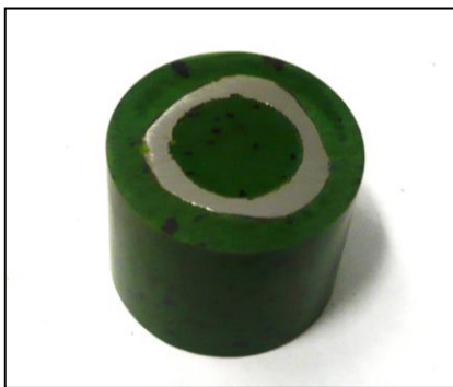
Figure 20: Mounted sample from tube A
