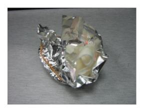
Figure 4.11: Ruptured PS cup at 125°C.
