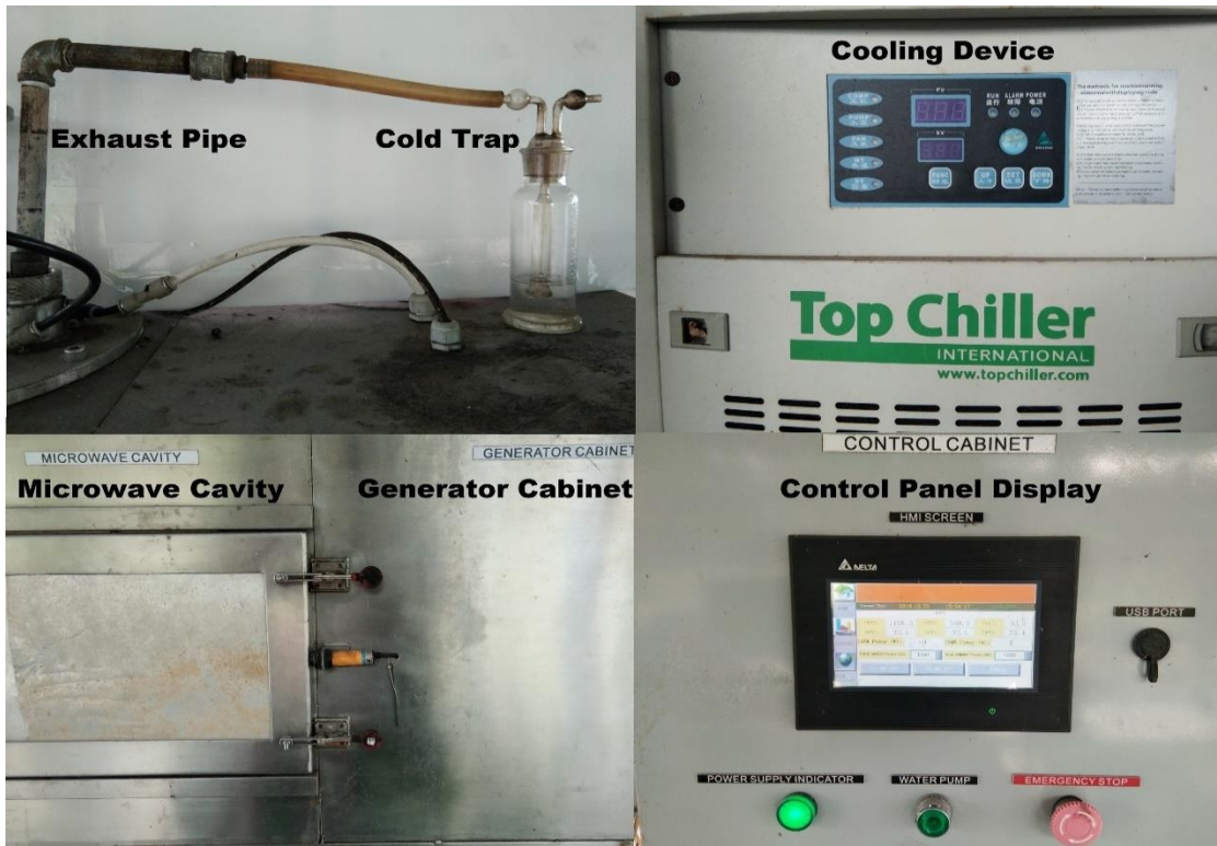
(B) Close-up view integrated with cooling device (placed backside of control cabinet)
