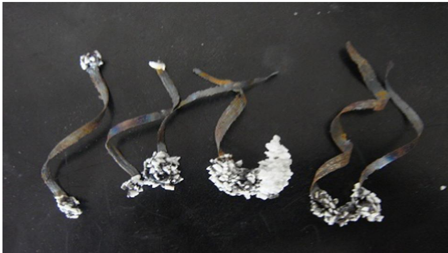
Figure 2.2: Morphology of the metal strips after discharge [66]
