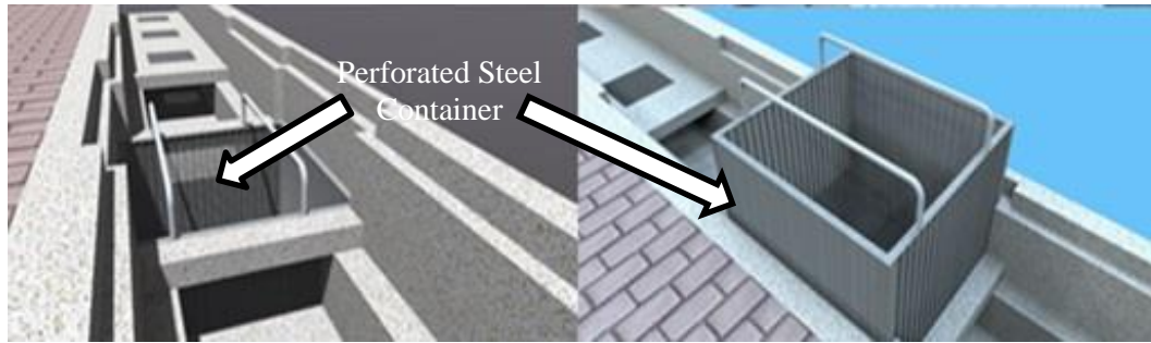
Figure 4.5: Top Plan of Clog Resistant Open Drain
