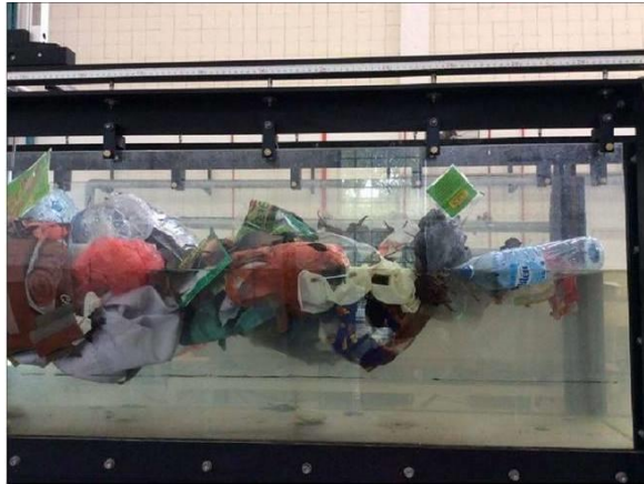
Figure 2.3: Litter clots in a model-drain
