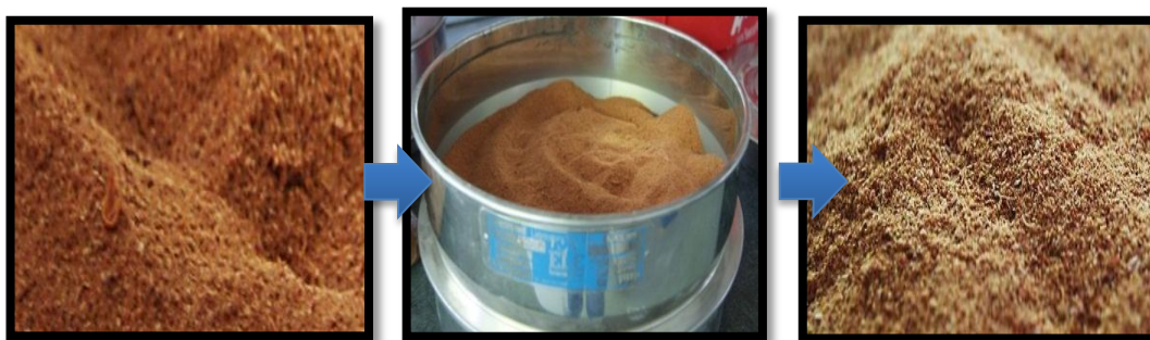
Figure 3.4: Wood flour preparation processes.
