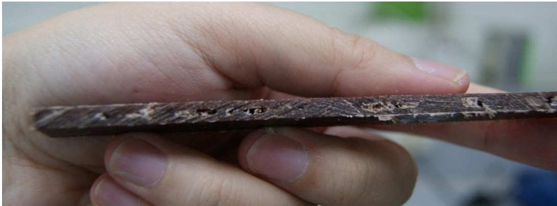
Figure 4.5: Visible voids in composite plate.
