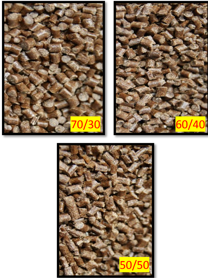
Figure 3.6: Samples after extrusion process.
