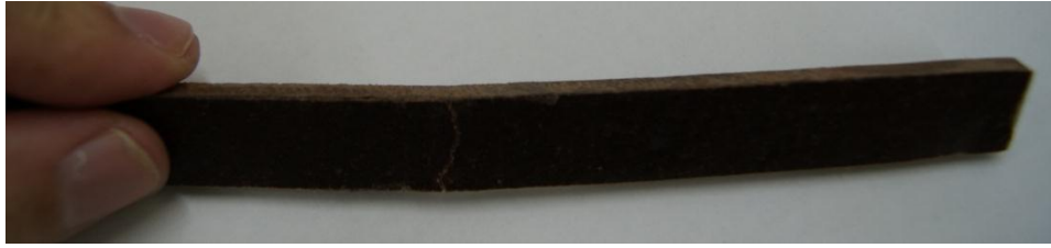
Figure 3.11: Bended or broken flexural specimen.
