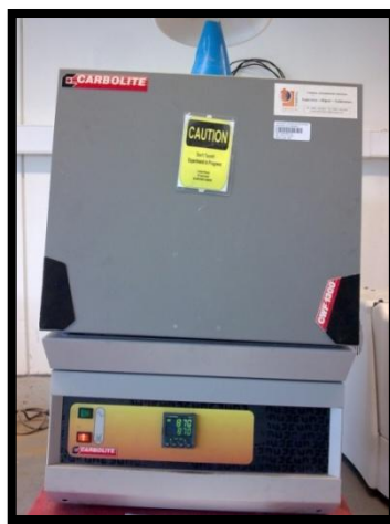
Figure 3.2: Furnace oven used for heat treatment
