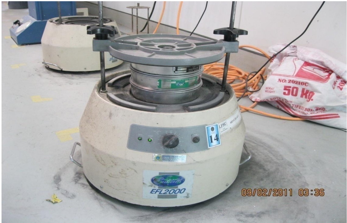
Figure 10: SIVE Shaker, Civil Engineering, Block13
