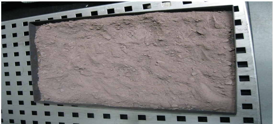
Figure 16: A mixture of raw materials ready for clinkering
