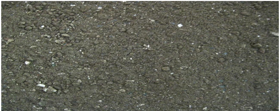
Figure 19: Portland cement clinker at temperature 1200\text{C}^{\circ}
