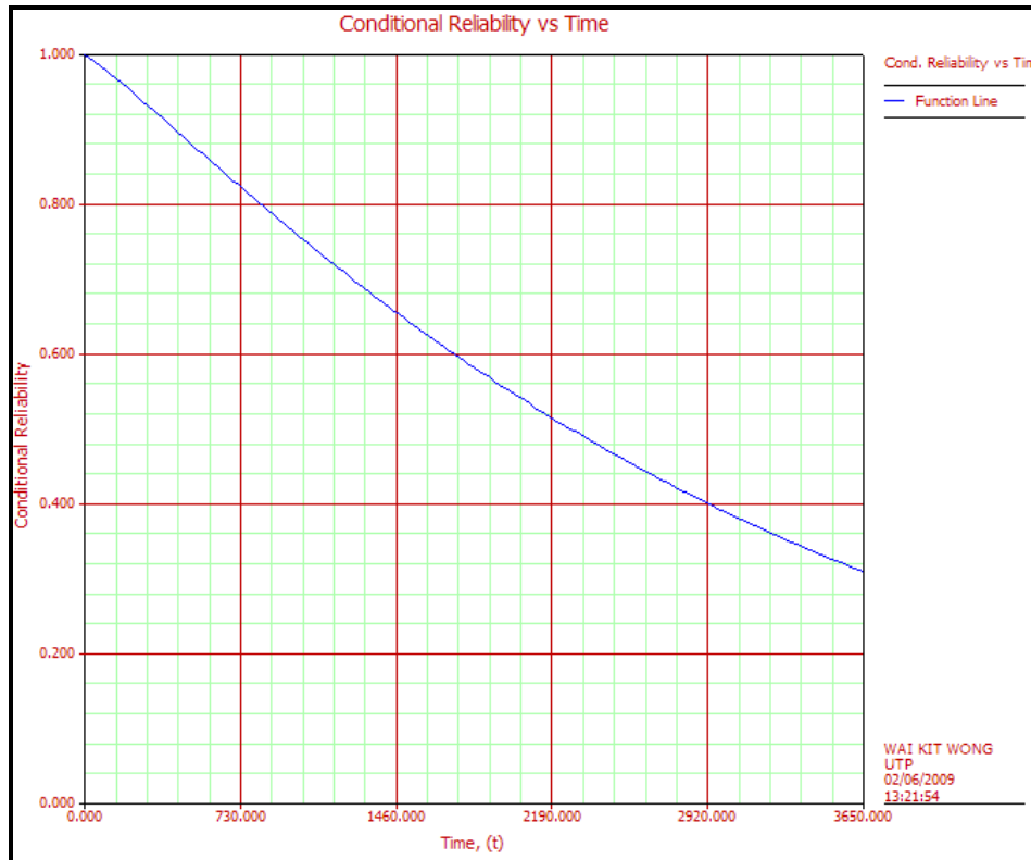
Figure 4.7: Conditional reliability vs. time of bearing
