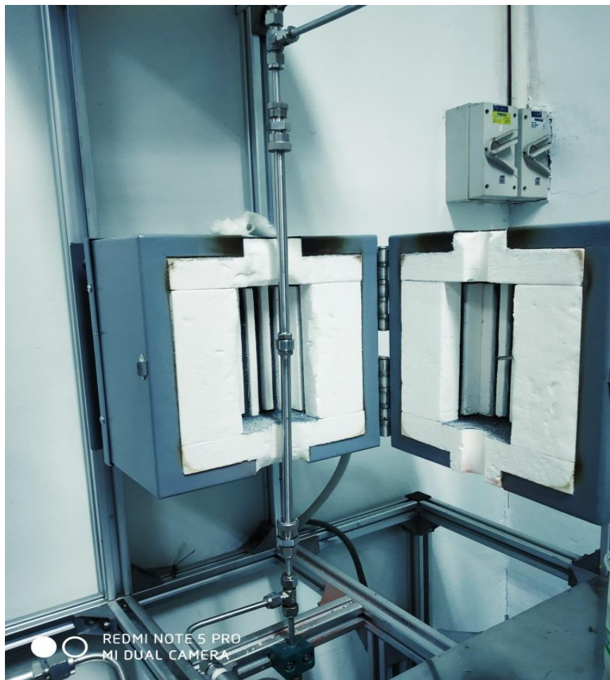
Figure A. 12. The fixed bed tubular reactor jacketed with furnace used for DRM reaction.
