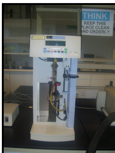
Figure 3.17 The Thermogravimetry apparatus (Brand Perkin Elmer model Pyris 1) used in this investigation
