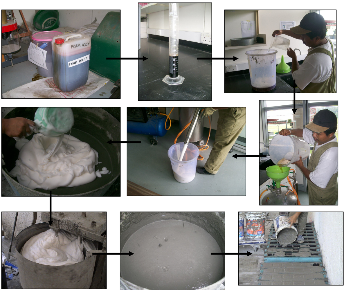
Figure 3.8 Foam production and casting processes
