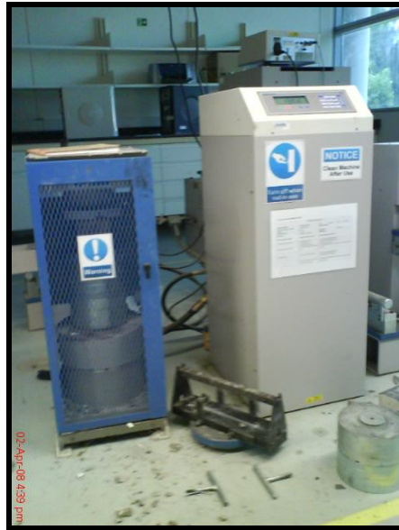
Figure 3.11 Compressive Testing Machine
