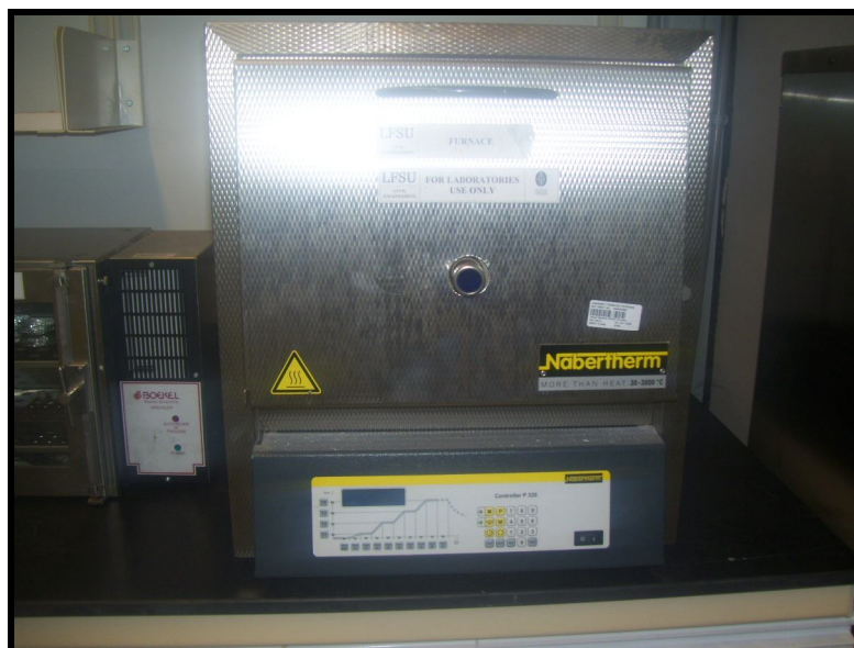
Figure 3.16 The electrical furnace apparatus (Nabertherm 30-3000°C) used in this study
