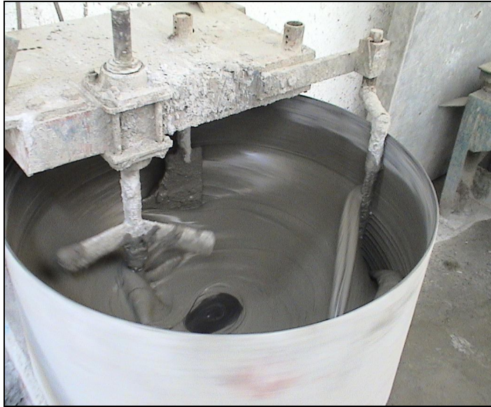
Figure 3.7 The preparation of mortar process as first process
