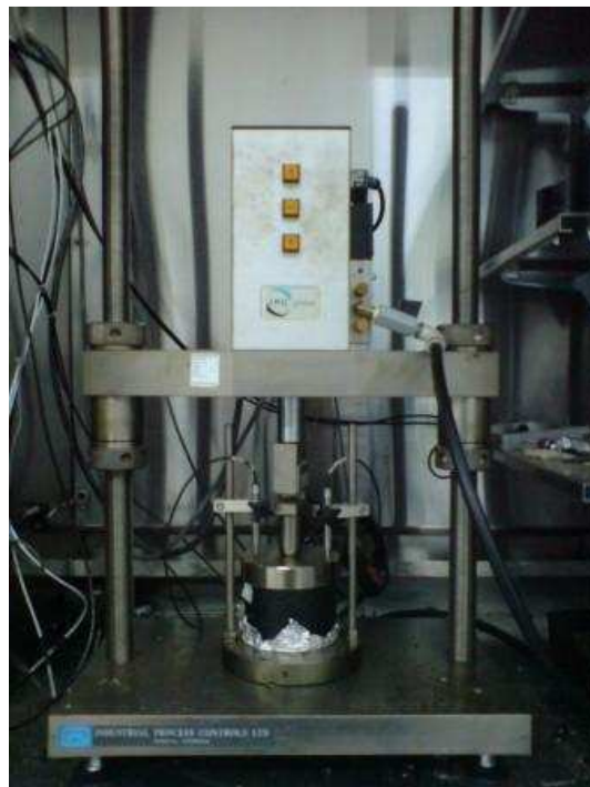
Figure 3.20 Dynamic Creep Test device
