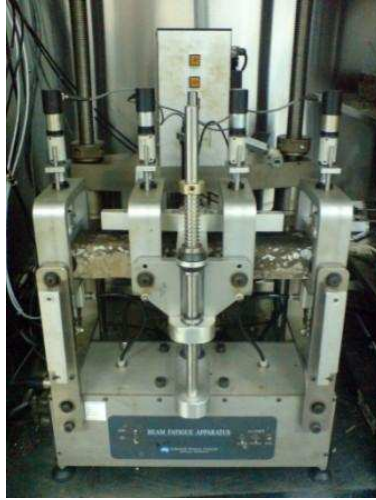
Figure 3.24 Beam Fatigue Test device
