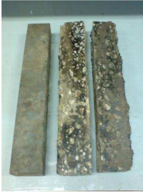
Figure 3.23 Beam Fatigue Test sample
