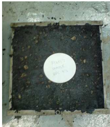
Figure 3.18 Wheel Tracking test sample
