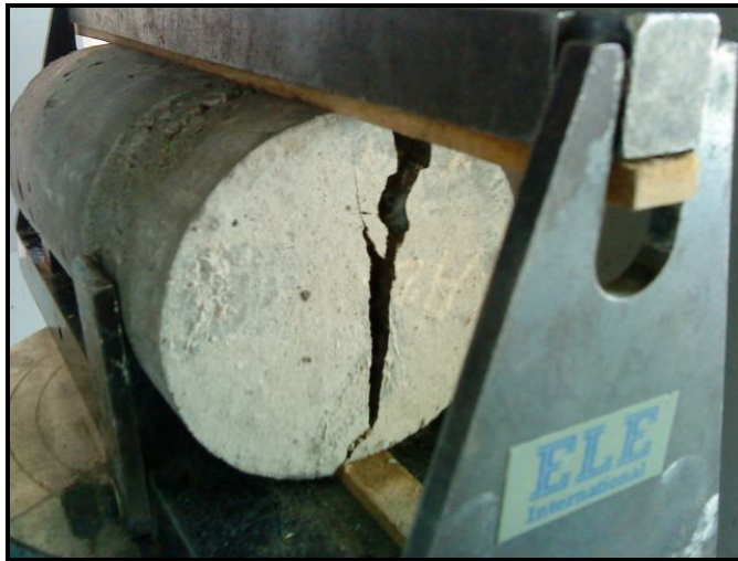
Figure 3.10: Split Cylinder Test
